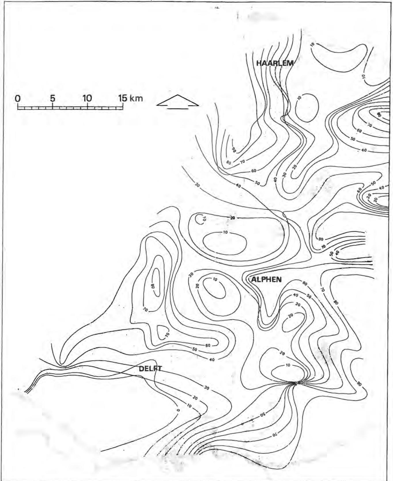
Fig. 2. Contour map of the depth (in m below sea level) of the 500 ppm chlorine concentration in the western part of the Netherlands
