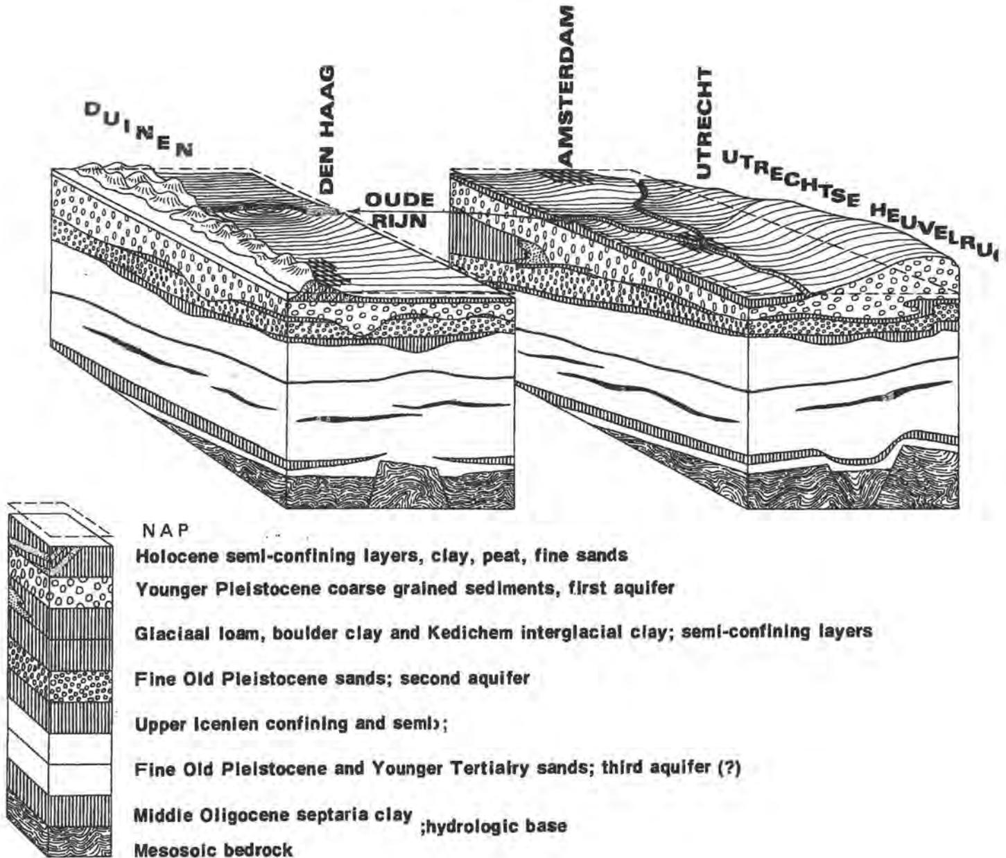
Fig. 1. Block diagram of the geological situation and conspectus of the hydrologically important layers found in the western part of the Netherlands
