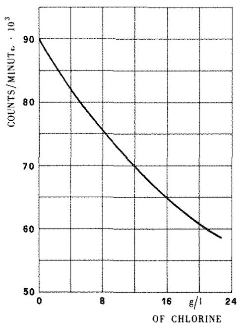
Fig. 2 - Calibration curve of the neutron probe for measuring the chlorine content of the ground water.
