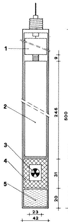
Fig. 1 - Scheme of the neutron probe for measuring the chlorine content of the ground water: 1) preamplifier; 2) counter; 3) neutron source; 4) lead shield; 5) rubber plug.
