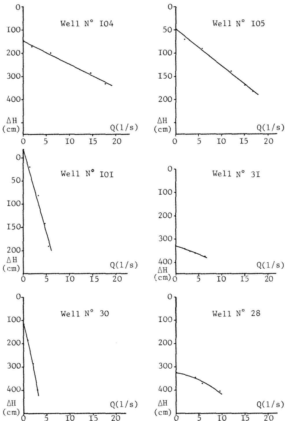
Fig. 4 - Characteristic curves with drawdown versus yield of some relevant wells in the delta of the Flumendosa (Nos. 28, 30, 31) and the Picocca (Nos. 101, 104, 105).
