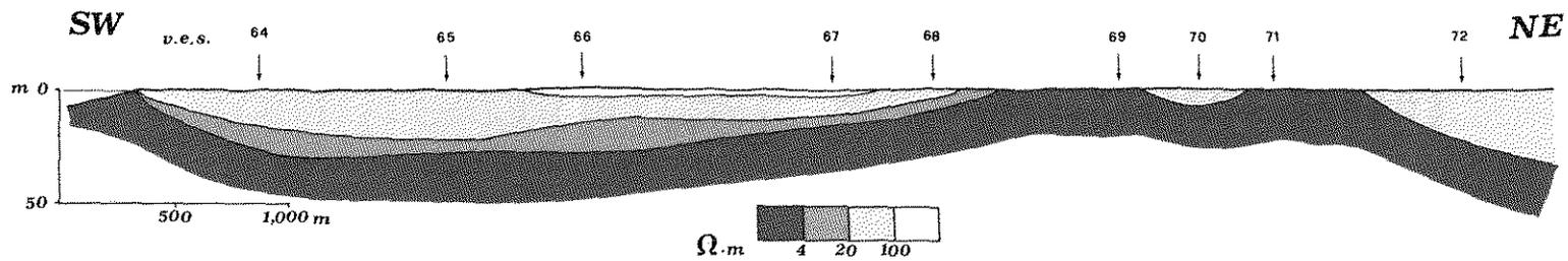
Fig. 5 - Electrical resistivity section of Versilia plain, 500 m south of Viareggio (from Geotecneco, 1975). Low resistivity values (less than 4  $\Omega \cdot m$ ) correspond to the salt water intrusion.
