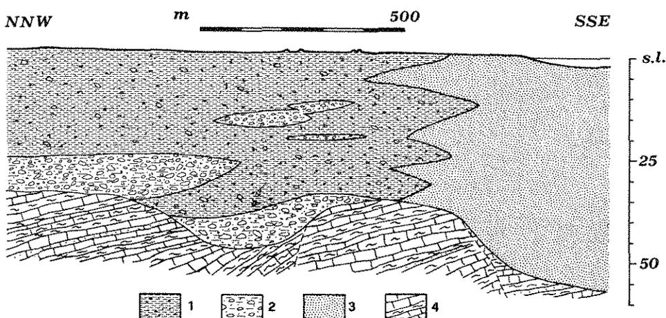
Fig. 6 - Geological section of Marina di Campo plain; 1: sandy silt; 2: gravel; 3: marine sands; 4: calcareous bedrock.
