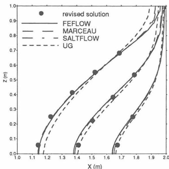
Fig. 1b Comparison of calculated isochlors with the revised solution obtained by Segol (1994). Isochlor values are 20%, 50% and 80% of seawater concentration.
