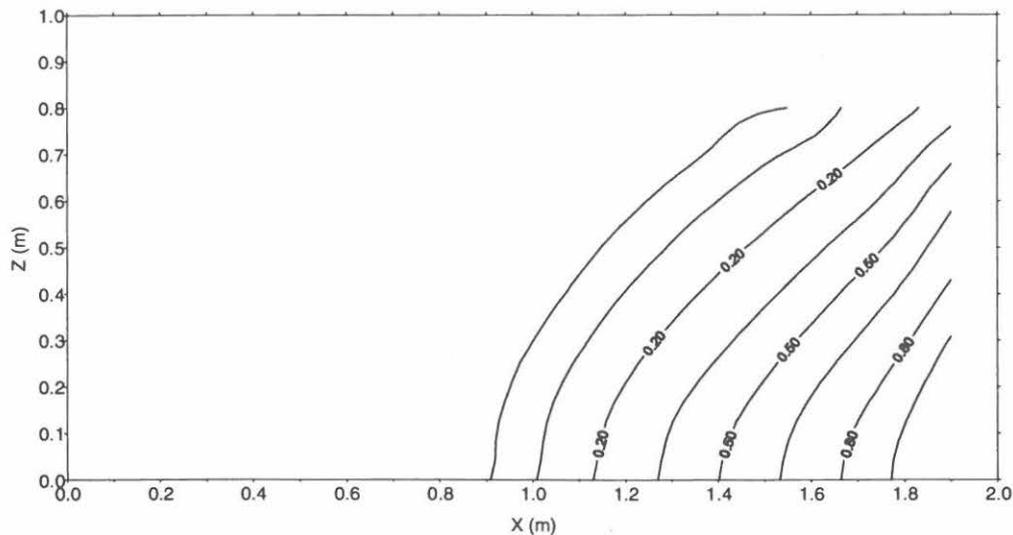
Fig. 1 Salt concentration isolines of the revised semi-analytic solution of the Henry problem (Segol, 1994); inflow from the left, fixed seawater concentration at the right, diffusion coefficient  $D = 18.86 \times 10^{-6} \text{ m}^2/\text{s}$ .
