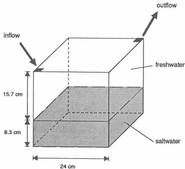
Fig. 6 Saltwater pool at the bottom of an impervious container with inflow and outflow at top corners.
