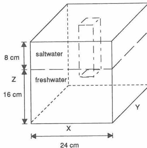
Fig. 2 Set-up for fingering experiments with unstable saltwater/freshwater layering.
