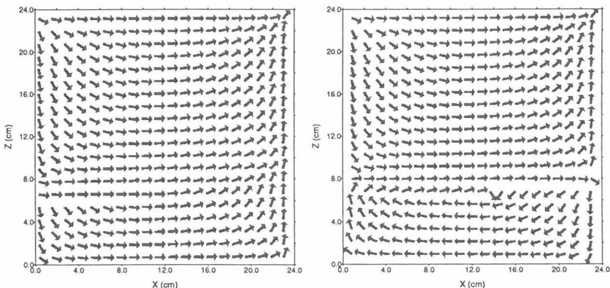
Fig. 7 Flow field in the centre  $xz$ -plane after 14 minutes, arrows show only direction of  $x,z$  components (a) initial salt concentration at the bottom is 100 g/l, total inflow/outflow is 0.1 l/min. (b) initially saturated brine (300 g/l) at the bottom, same inflow/outflow as in (a).
