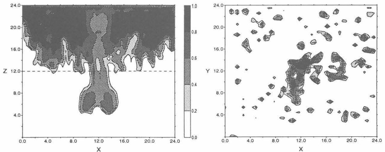
Fig. 3 Fingering of saltwater in unstable layering with central heterogeneity (a) Vertical centre plane, permeability ratio of 5.1, after 176 minutes; (b) Horizontal plane, permeability ratio of 3.2, 4 cm below initial interface as indicated in 3a (dotted line), after 166 minutes.
