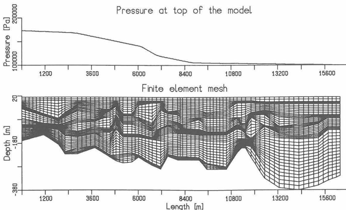
Fig. 3. Finite element mesh and pressure at top of the model.
