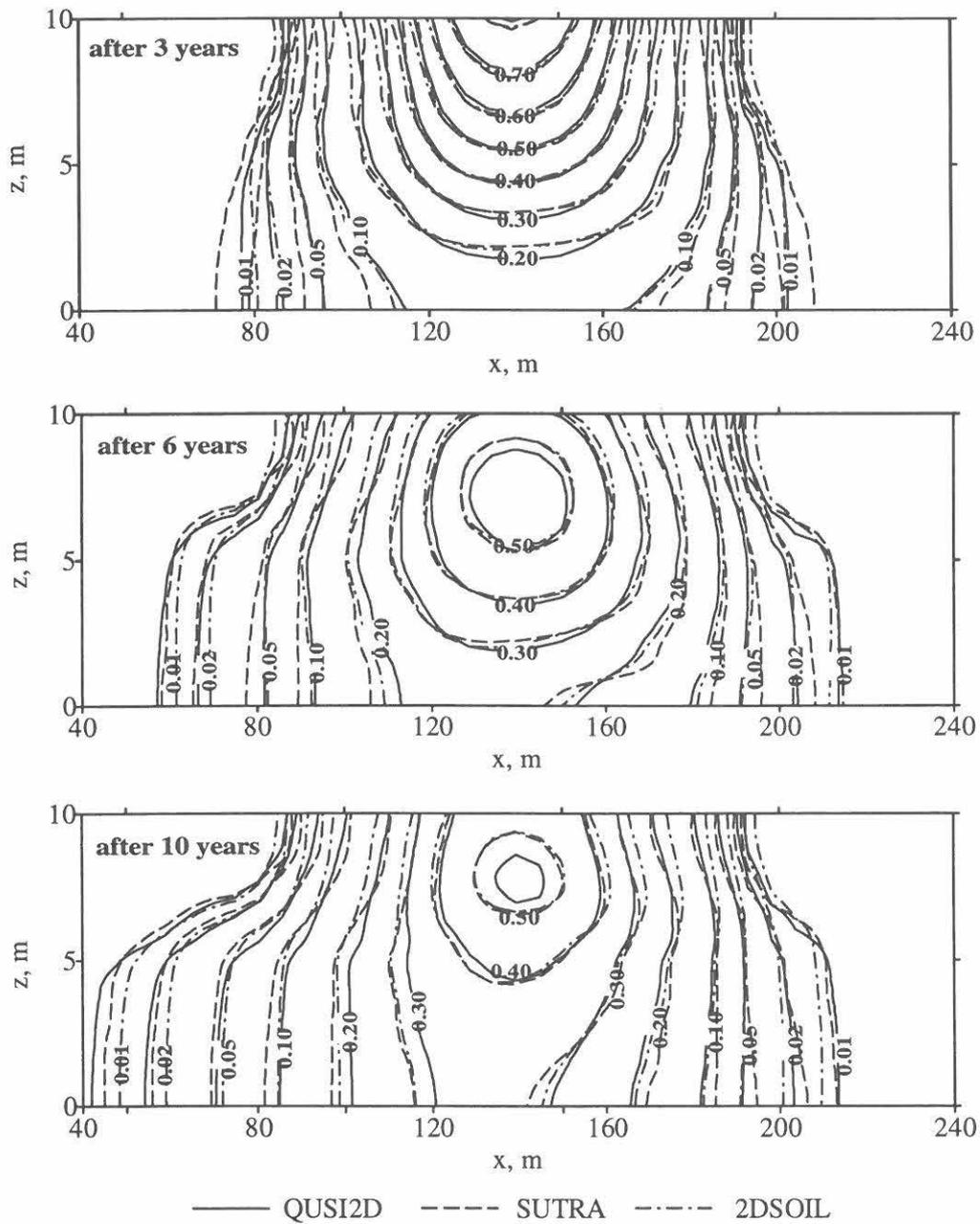
Figure 3. Contours of the solute concentration during infiltration from the soil surface.
