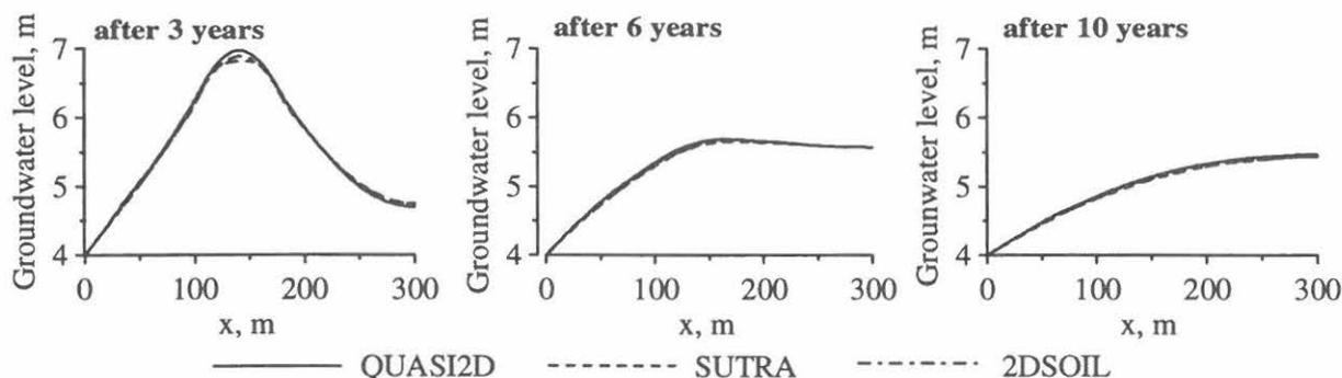
Figure 2. Groundwater level during infiltration from the soil surface.
