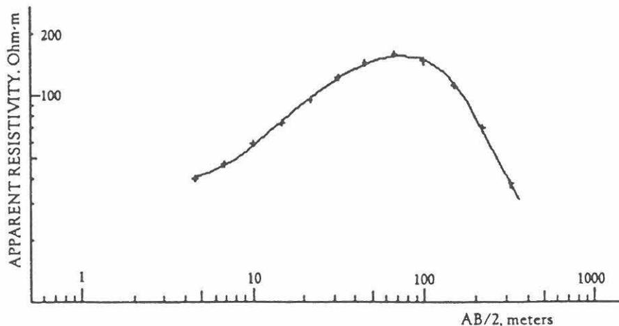
Fig. 5 Resistivity as function of depth from electrical sounding in Håslöv.
