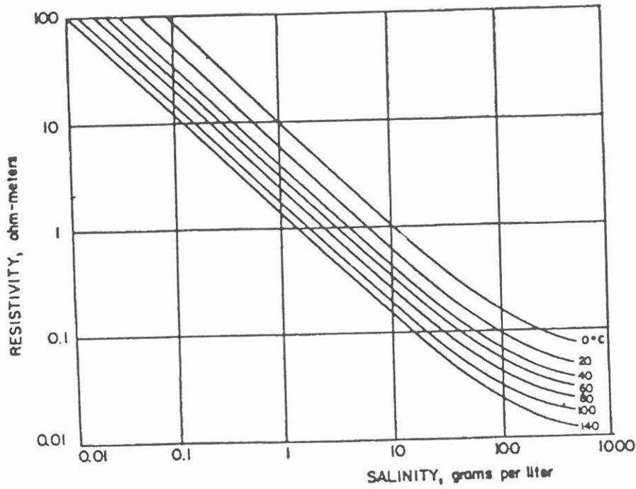
Fig. 3 Resistivity of solutions of sodium chloride as a function of concentration and temperature.
