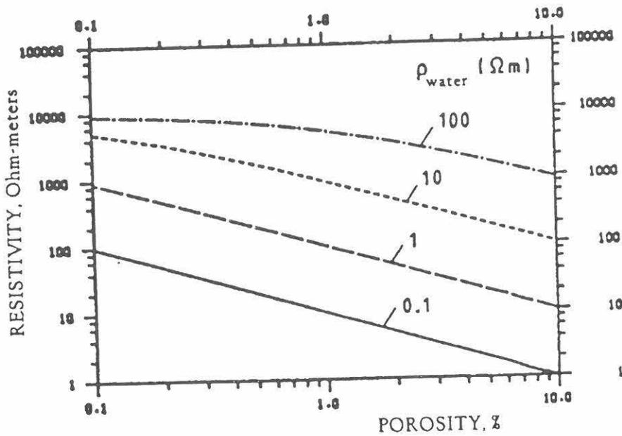
Fig. 4 Resistivity of the bedrock as function of porosity and the resistivity of the electrolyte.
