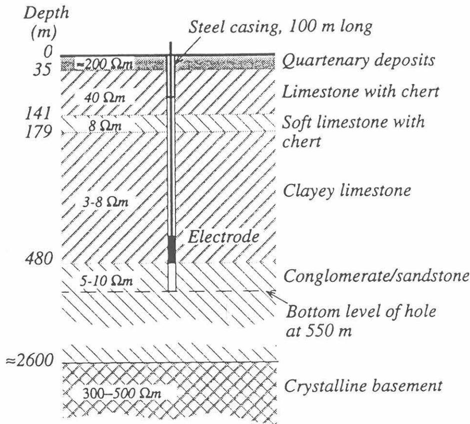
Fig. 6 Resistivities, earth layers and location of the electrode in the bore hole.
