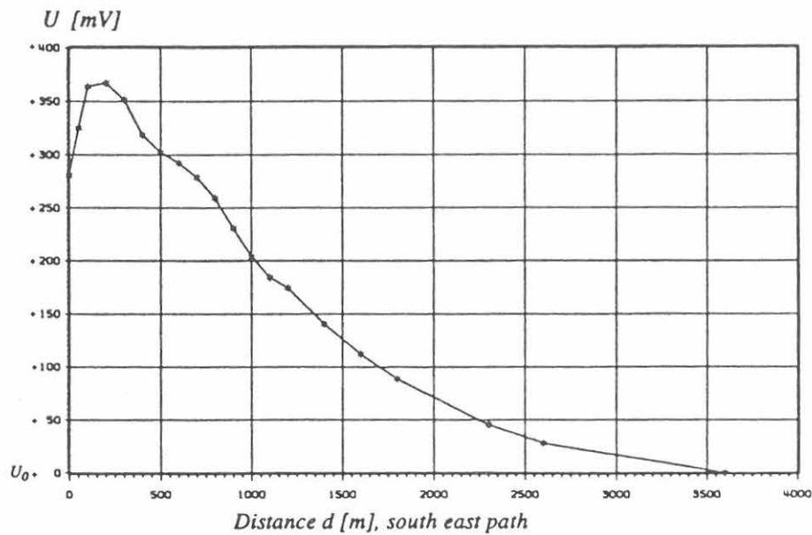
Fig. 8 Measured potential distribution referred to 350 A.  $U_0$ =reference voltage at 3.6 km.
