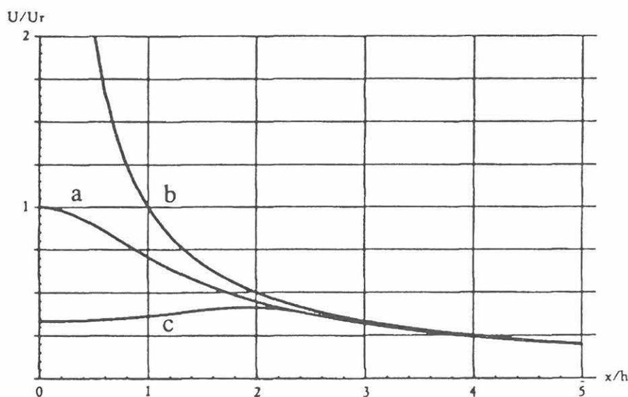
Fig. 7 Potential distributions at the surface of a homogeneous earth.  $x$ =horizontal distance,  $U_r$ =maximum voltage in case a.
