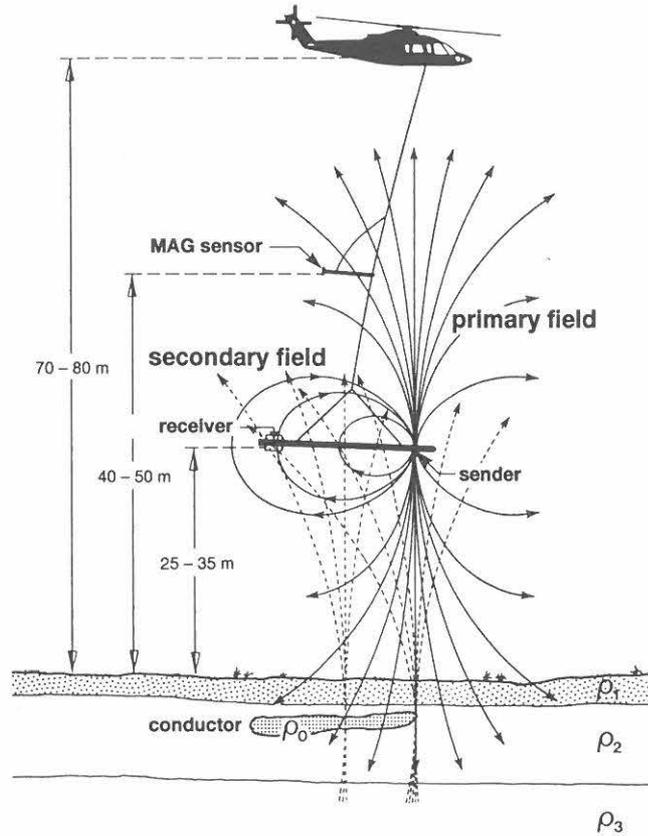
Fig. 1: Sikorsky S 76 B helicopter carrying the EM and magnetometer sensors at the indicated elevations above ground. Geometry of the transmitted primary magnetic field (dipole field) inducing currents in the conductive parts of the ground. Sketch of the secondary magnetic fields of these currents flowing in the three layers ( $\rho_1$ ,  $\rho_2$ ,  $\rho_3$ ) and the conductor ( $\rho_0$ ); a small portion of the secondary field passes through the receiver coil.
