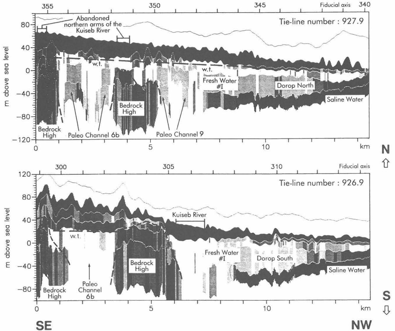
Fig. 5: VRS for SE–NW tie-lines showing the Dorop aquifer (see Figs. 3 & 4), the underlying "saline wedge", and the bordering bedrock high SE of Dorop. Another freshwater aquifer (PC 6b) can be identified between bedrock flanks of higher resistivity.
