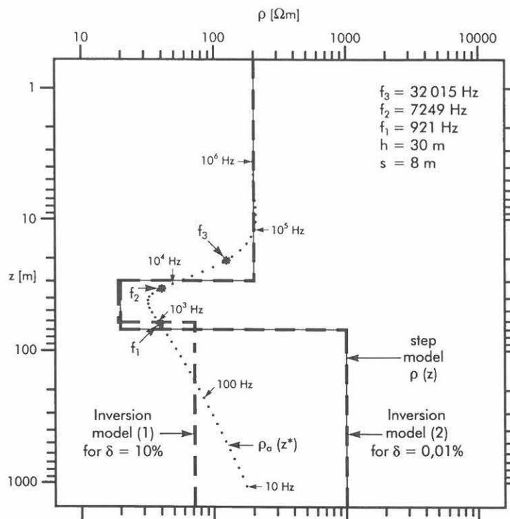
Fig. 2:  $\rho/z$  diagram showing resistivities  $\rho$  and thicknesses  $d$  of a three-layer model  $\rho(z)$ , where  $\rho_1 = 200$ ,  $\rho_2 = 20$ ,  $\rho_3 = 1000$   $\Omega\text{m}$ ,  $d_1 = 30$ ,  $d_2 = 40$  m, and the results of different inversion methods:
