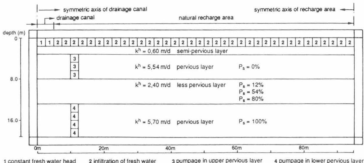
Figure 6. Geometry and subsoil parameters of the modeled cross-section
