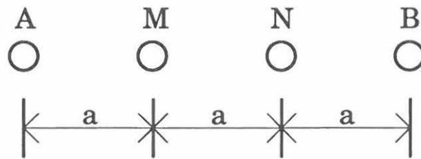
Figure 1. *The Wenner electrode configuration.*
