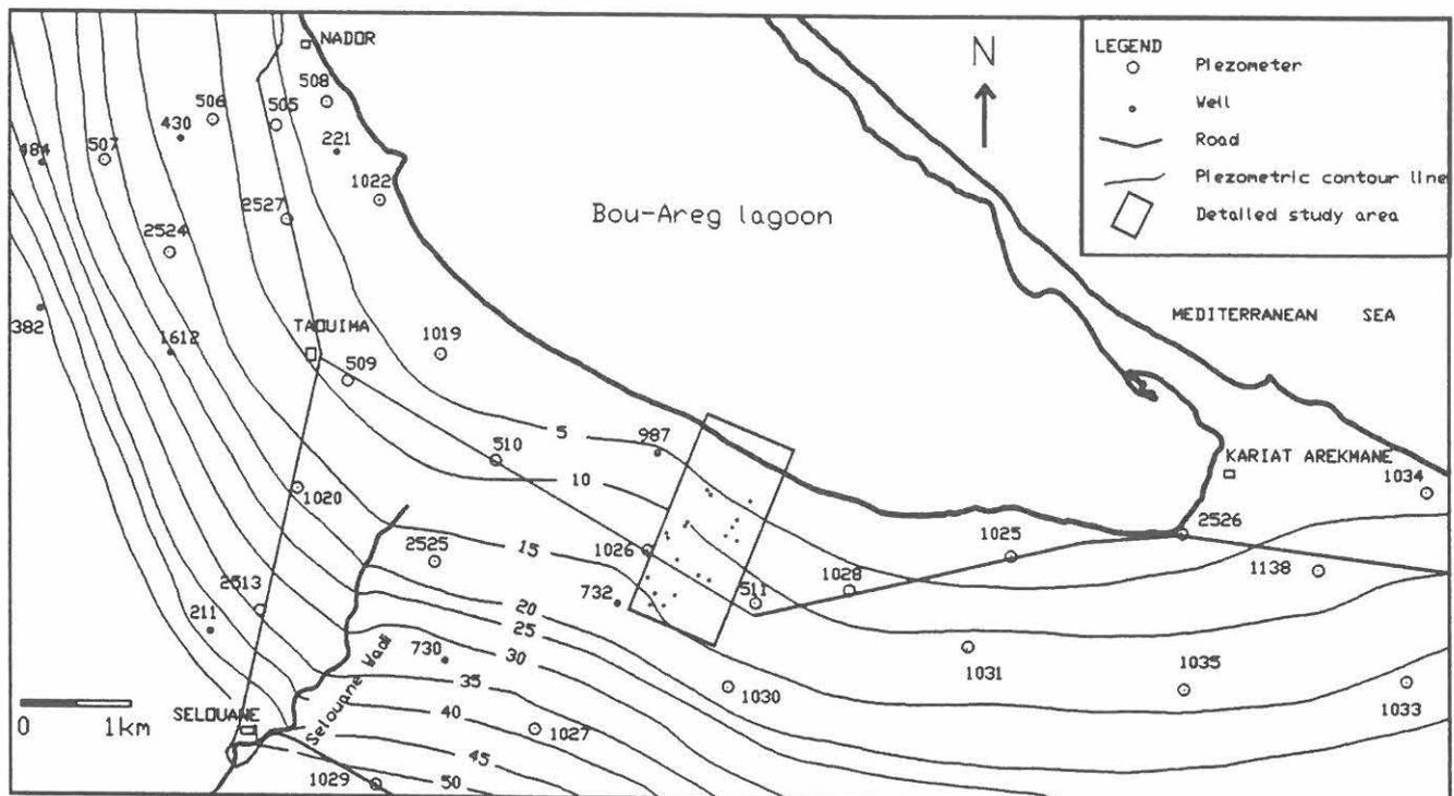
Fig. 9 - Location of observation wells and piezometric surface of Bou-Areg aquifer.
