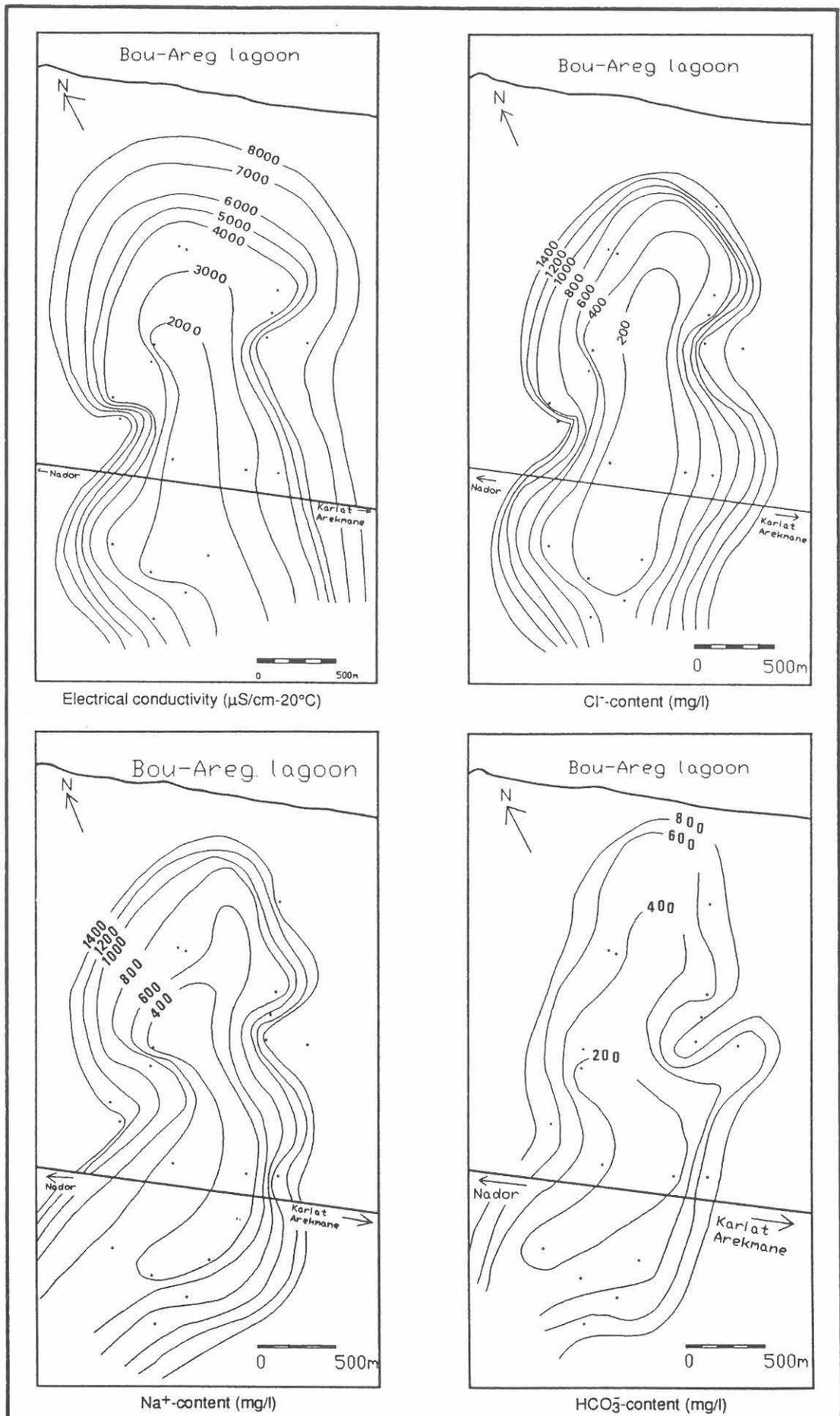
Fig. 12 - Chemical parameters in groundwater of detailed study area in November 1995 (Bou-Areg aquifer).
