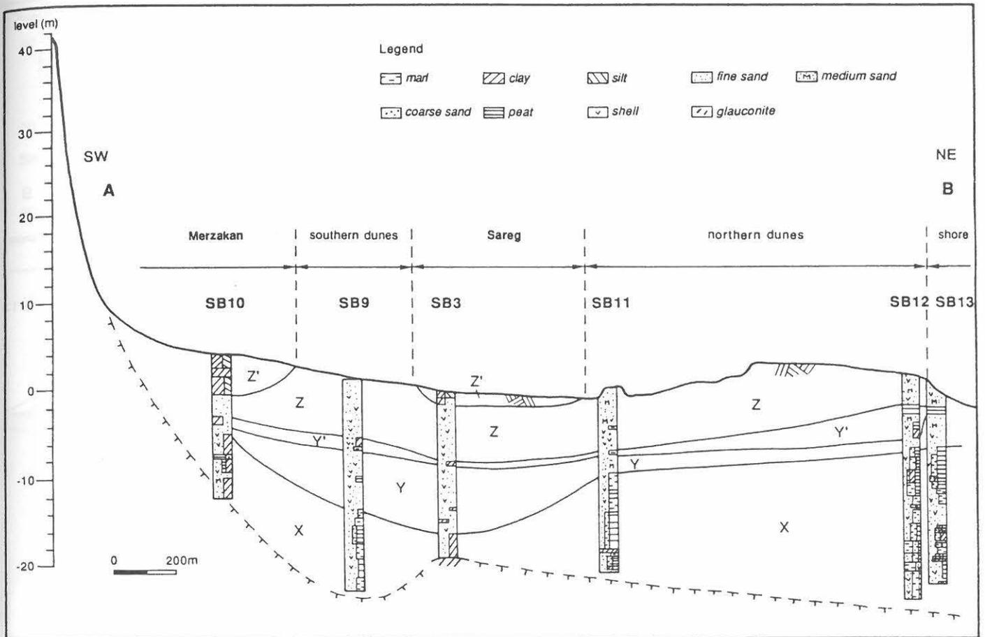
Fig. 3 - Lithology and hydrogeological structure in profile AB through the coastal plain of Saidia.
