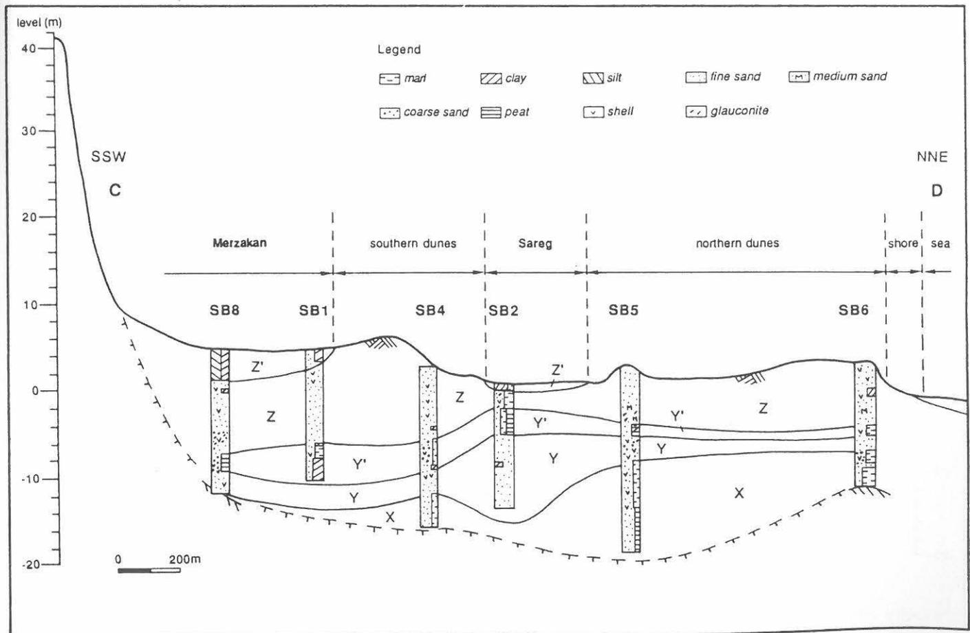
Fig. 4 - Lithology and hydrogeological structure in profile CD through the coastal plain of Saidia.
