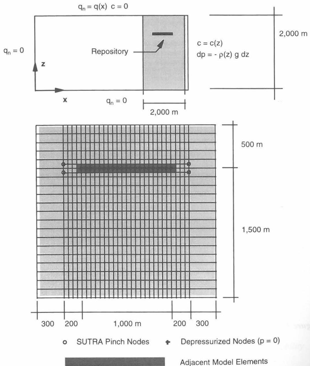
**Figure 6** Finite-element discretization for simulation of saline intrusion to a repository. The complete mesh consists of 1,528 nodes and 1,436 elements.
