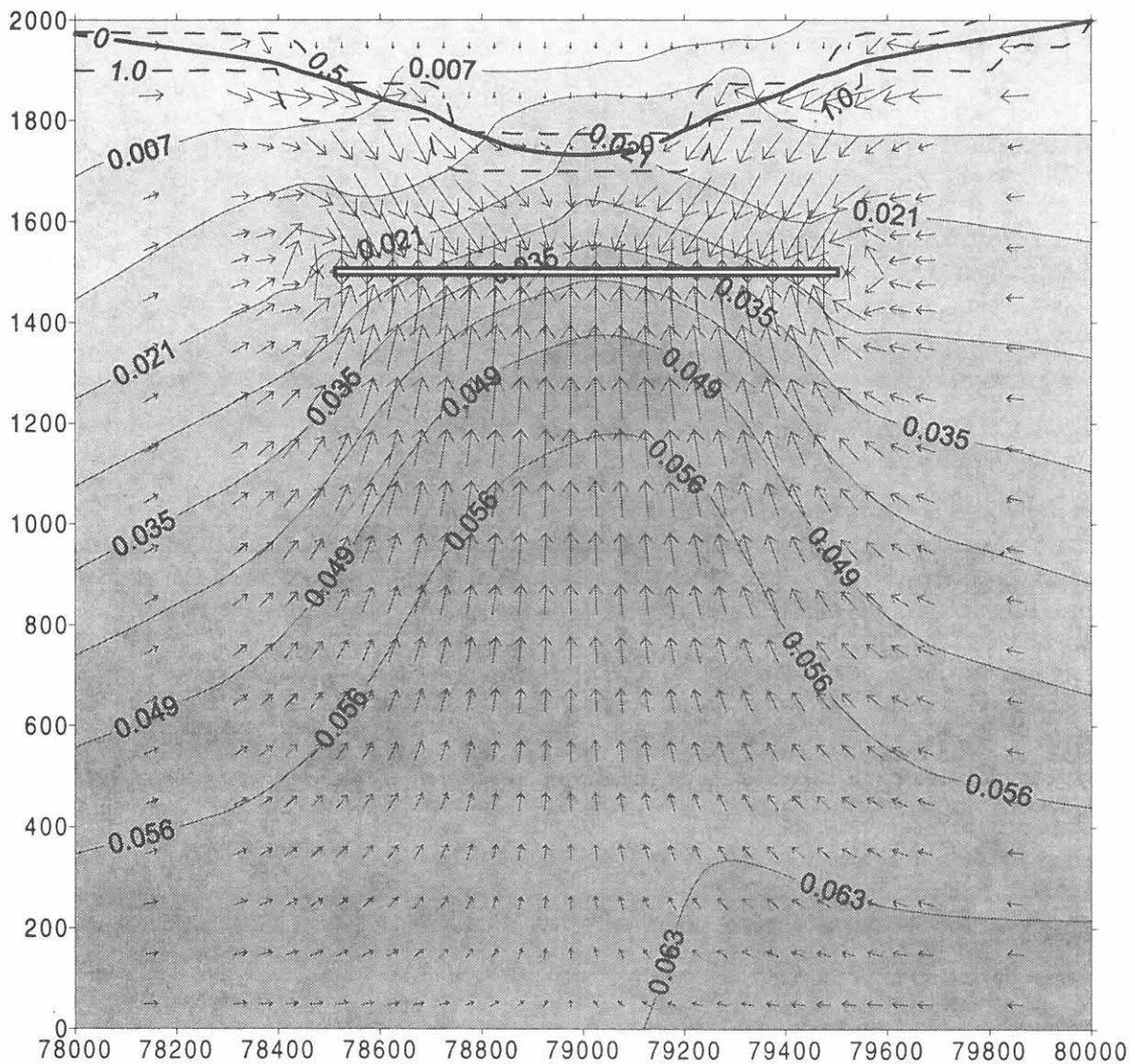
**Figure 9** Situation after 50 years of dewatering of case B (the permeability of the model elements adjacent to the repository is decreased 2 orders of magnitude with regard to case A).
