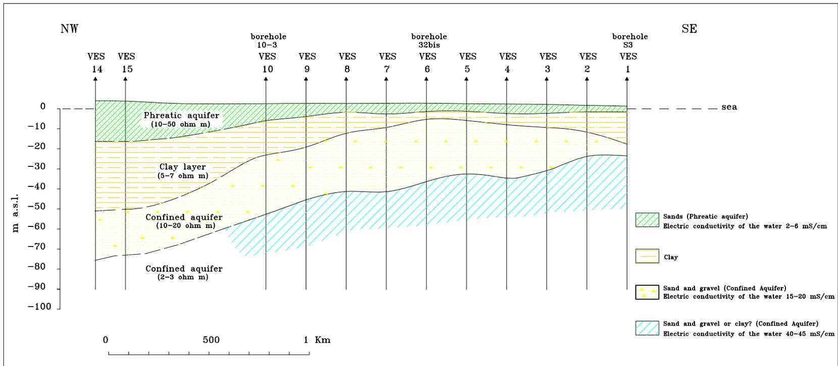
Figure 3 – Hydrogeological interpretation based on geognostic drillings and vertical electrical soundings
