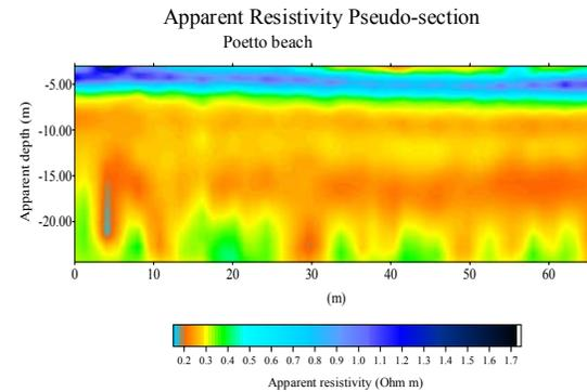
Fig.4 – Apparent resistivity pseudosection showing different conductive layers
