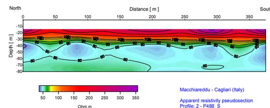
Fig.7- Apparent resistivity pseudosection in a profile parallel to salt-works.
