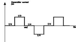
Fig.1- Transmitter current waveform
