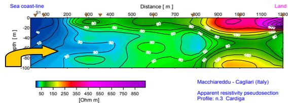
fig.5- Apparent resistivity pseudosection showing the salt water intrusion far from the coastal line.
