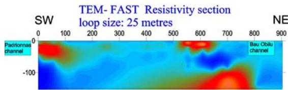
Fig.8a,b- Resistivity section obtained respectively from a TEM FAST survey and a TEM survey.
