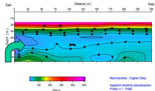
Fig. 6- Apparent resistivity pseudosection in a profile perpendicular to salt-works showing salt water intrusion and the "spray" effect
