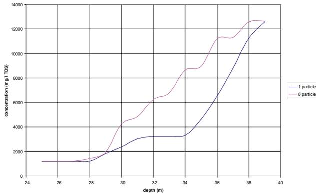
**Figure 3 Difference in upconing curve for 1 particle and 8 particles per cell after three days of pumping**
