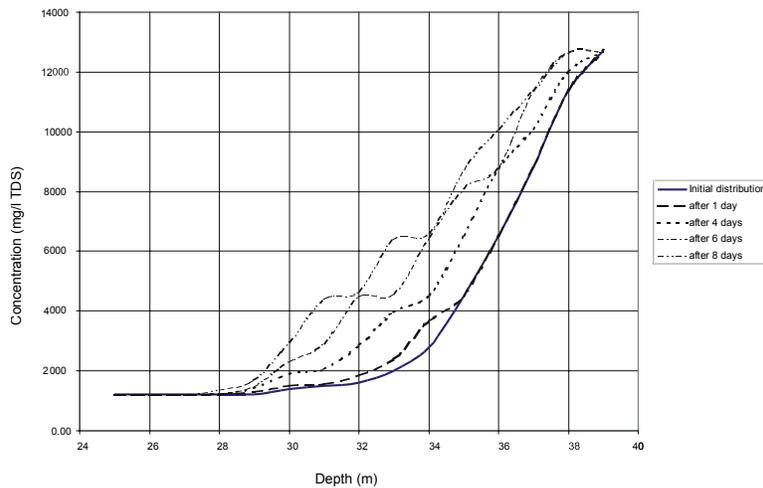
**Figure 4 Result of the forward run. Upconing of the transition zone at different moments in time**
