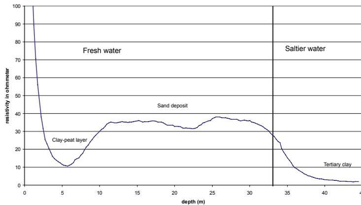
**Figure 1 LN resistivity profile of a well in the central part of the Belgian Coastal Plain with indication of the fresh-salt water transition zone**
