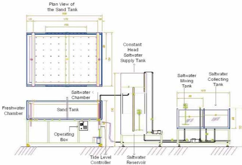
Figure 2. Drawing of the sand tank for the three-dimensional experiments.
