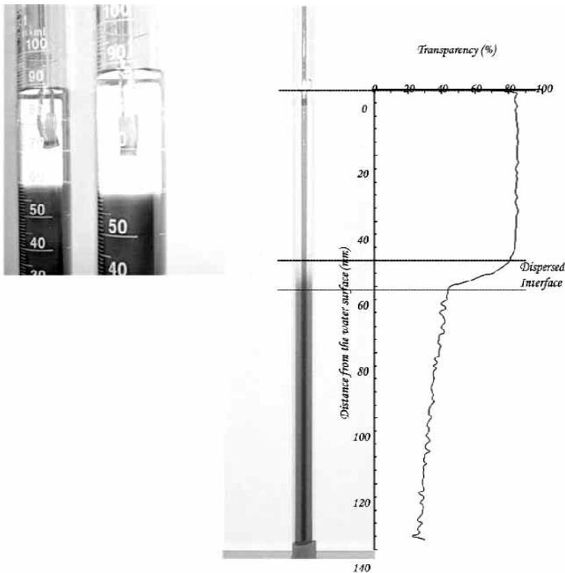
**Figure 4.** Detection of the interface using a sample column of water.
