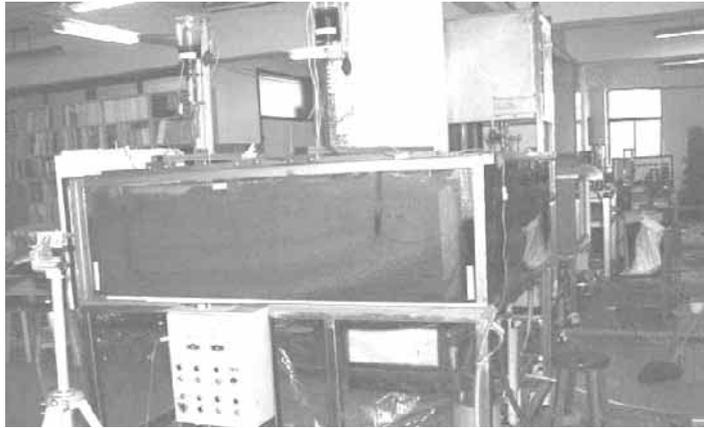
**Figure 3.** Sand tank for the three-dimensional experiments.
