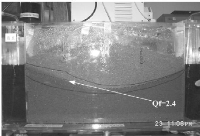
**Figure 6.** (a) Schematic diagram of the pumping scenario. (b) Shift in the interface position due to pumping.
