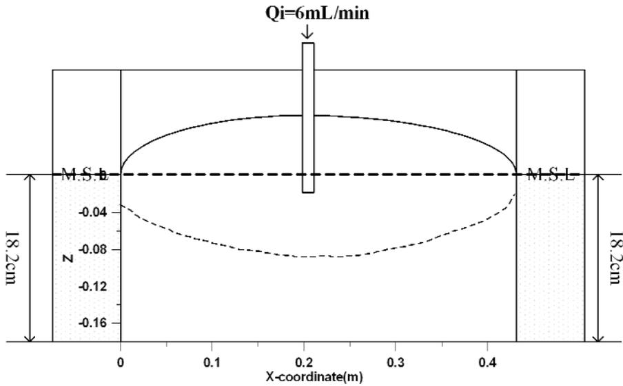
Figure 1. Sand tank for the cross-sectional experiment.
