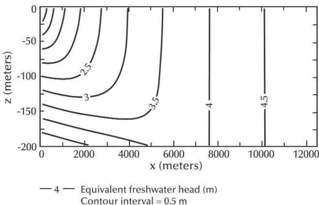
**Figure 3.** Equivalent freshwater heads calculated using SEAWAT for solution one.
