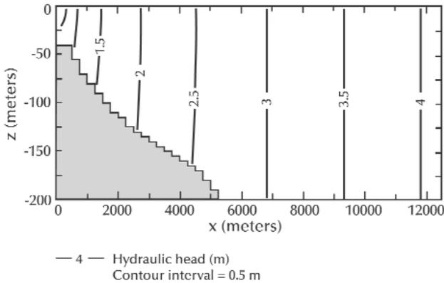
**Figure 7.** Hydraulic heads calculated using MODFLOW for solution five (inactive cells to represent interface and equivalent freshwater head  $h_{fw}$  at coastal boundary).
