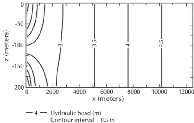
**Figure 6.** Hydraulic heads calculated using MODFLOW for solution four (inactive cells to represent interface and  $h_{sw} = 0$  at coastal boundary).
