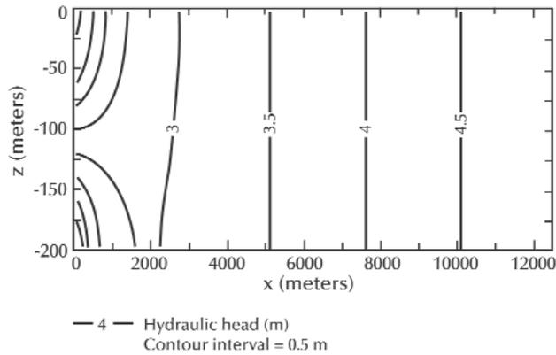
**Figure 5.** Hydraulic heads calculated using MODFLOW for solution three (equivalent freshwater head  $h_{fw}$  at coastal boundary).
