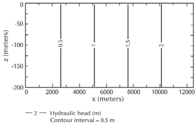
**Figure 4.** Hydraulic heads calculated using MODFLOW for solution two ( $h_{sw} = 0$  at coastal boundary).
