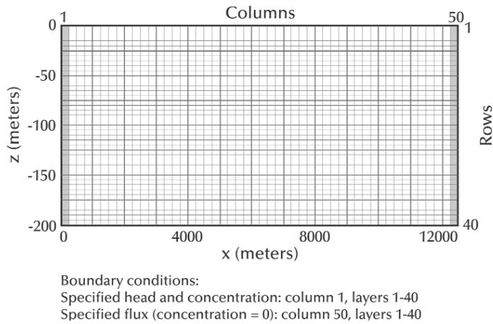
**Figure 1.** Finite-difference grid used for numerical experiments.
