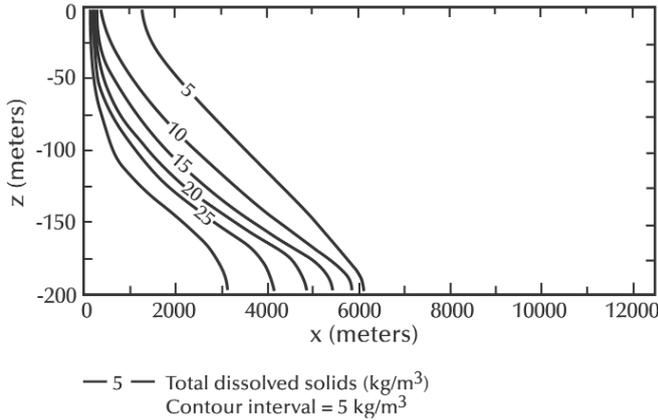
**Figure 2.** TDS concentrations calculated using SEAWAT for solution one.
