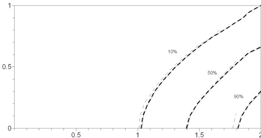
**Figure 2.** Comparison between TRANSDENS (solid line, identical for both Newton-Raphson and Picard methods), SUTRA (thick dashed line) and the semi-analytical solution given by Segol (1994) (thin dashed line). Isolines corresponding to 90%, 50% and 10% of mixing between freshwater and seawater are shown.
