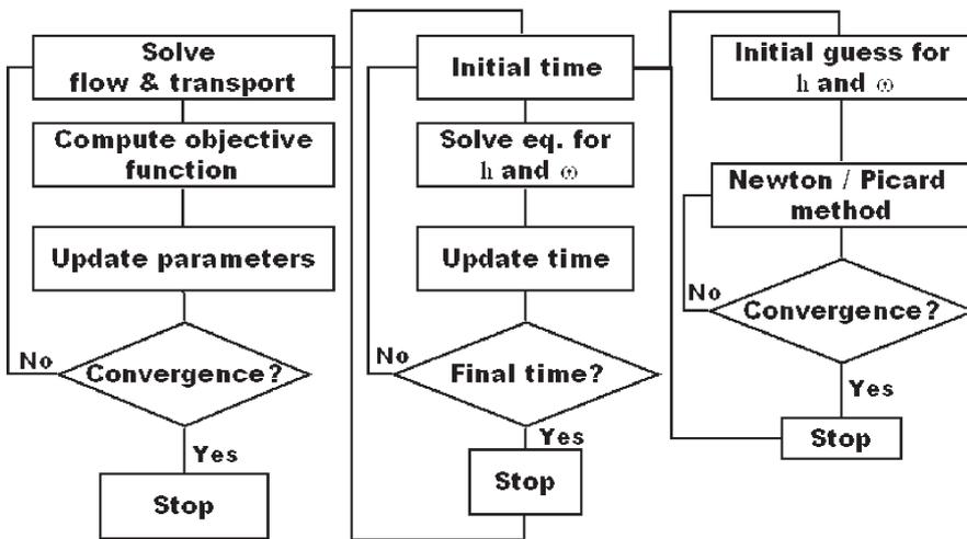
**Figure 1.** Automatic parameter calibration process showing the inner loops corresponding to the solution of the non-linear coupled flow and transport equations ( $h$  stands for equivalent fresh water head and  $w$  for solute mass fraction).
