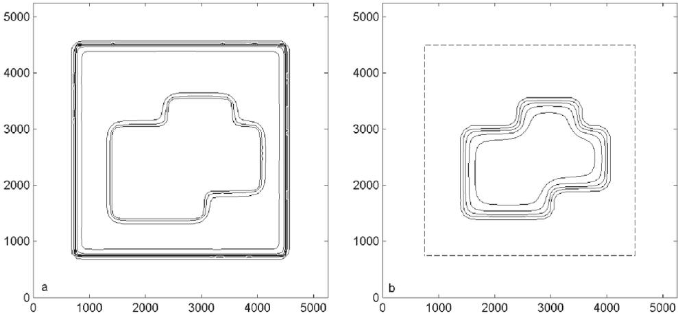
**Figure 4.** Contours of the elevation of the steady interface position in (a) aquifer 2, and (b) aquifer 3
