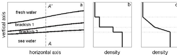
**Figure 1.** (a) Conceptual model with three surfaces, (b) density distribution of stratified flow, (c) density distribution of variable density flow
