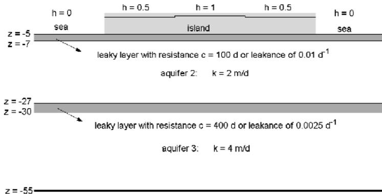
**Figure 2.** Schematic cross-section of the island aquifer system
