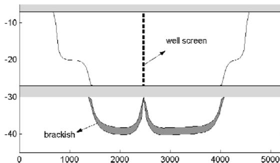
**Figure 7.** Position of an initially 2 m thick brackish zone after 20 years of pumping along cross-section  $B-B'$
