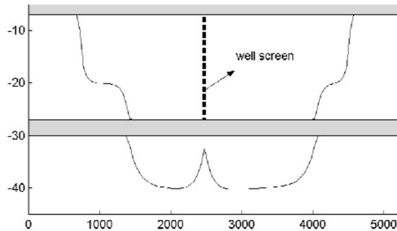
**Figure 6.** Position of the interface after 20 years of pumping along cross-section  $B-B'$
