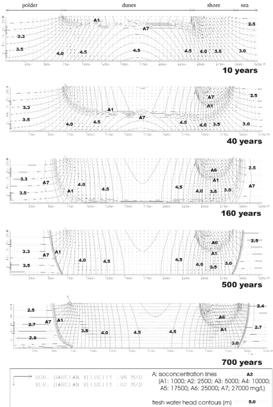
**Figure 2.** Evolution of water quality distribution in the polder, dunes and under the shore and sea. The simulation starts in 1300 AD and 500 year simulation time corresponds with 1800 AD, 700 years with 2000 AD or the current situation. Lines of constant fresh-water head are indicated together with isoconcentration lines and groundwater flow and its velocity using arrows.
