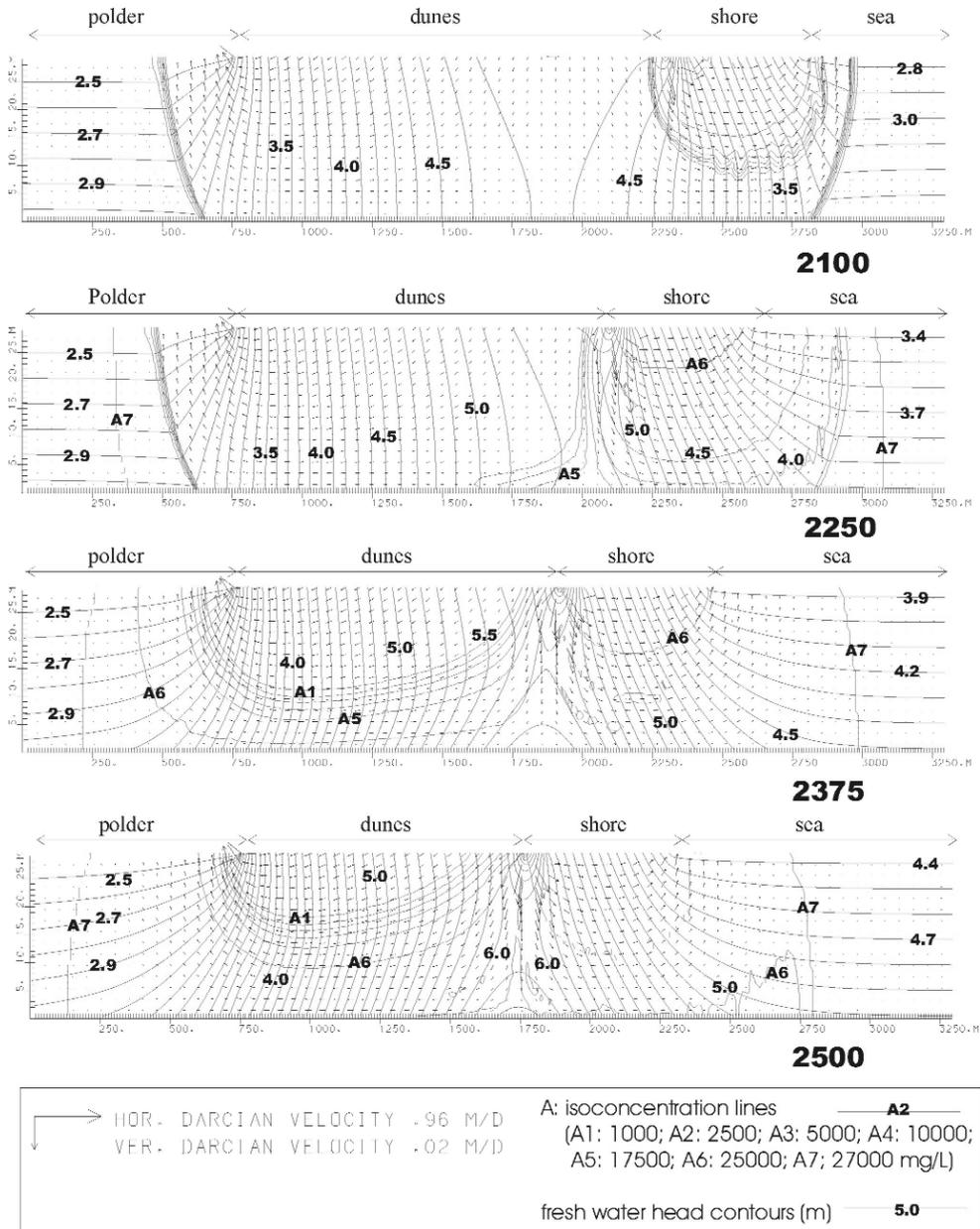
**Figure 5.** Water quality evolution, fresh-water head and flow under the shore, dunes and polder along the French-Belgian border with a sea level rise of 0.4 m and in the case the coastline is retreating. This is shown for 2100 AD, 2250 AD, 2375 AD and 2500 AD. Lines of constant fresh-water head are indicated together with isoconcentration lines and groundwater flow and its velocity using arrows.
