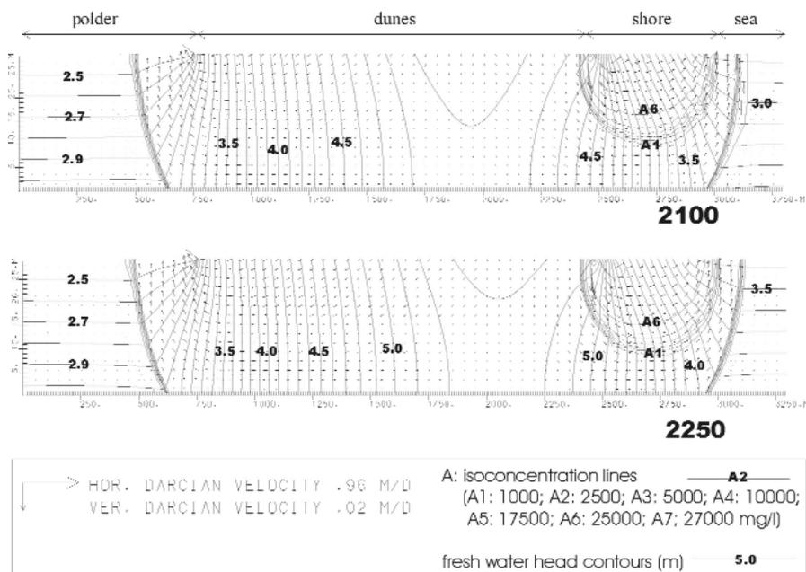
**Figure 4.** Water quality evolution, fresh-water head and flow under the shore, dunes and polder along the French-Belgian border with a sea level rise of 0.4 m and in the case a dike is present and the shore is heightened. This is shown for 2100 AD, and 2250 AD. Lines of constant fresh-water head are indicated together with isoconcentration lines and groundwater flow and its velocity using arrows.
