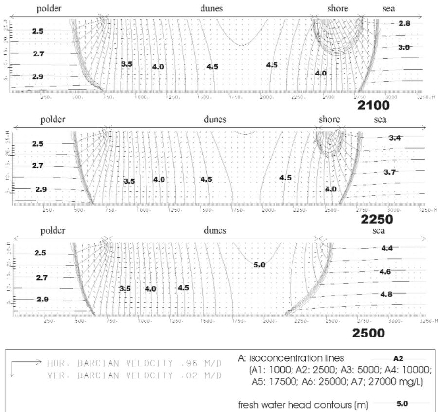
**Figure 3.** Water quality evolution, fresh-water head and flow under the shore, dunes and polder along the French-Belgian border with a sea level rise of 0.4 m and in the case a coastal defence is present. This is shown for 2100 AD, 2250 AD and 2500 AD. Lines of constant fresh-water head are indicated together with isoconcentration lines and groundwater flow and its velocity using arrows.
