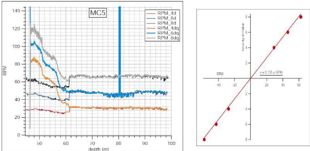
**Figure 6.** Impeller flow-meter recording for different cable speed runs down without and with pumping (q) and calibration of RPM with velocity.
