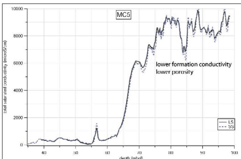
**Figure 9.** The formation conductivity recorded in borehole MC5, all other boreholes have similar shapes and peaks.
