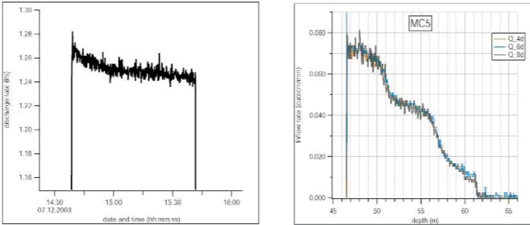
Figure 7. Calculated inflow rates for MC5 and recorded discharge rate during testing (left).
