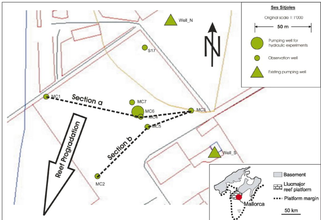
**Figure 1.** Ses-Sitjoles test site, location and drilling distribution.
