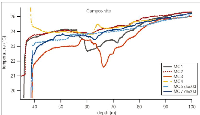
Figure 8. Temperature profile for all boreholes in Campos; MC3 has the largest anomaly at 65 m depth.
