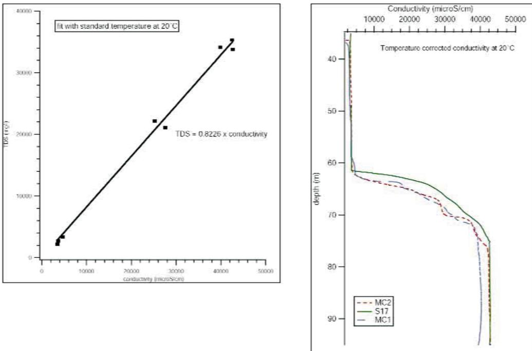
**Figure 10.** Conductivity profile for a selection of boreholes and the empirically derived relationship between measured conductivity and TDS.
