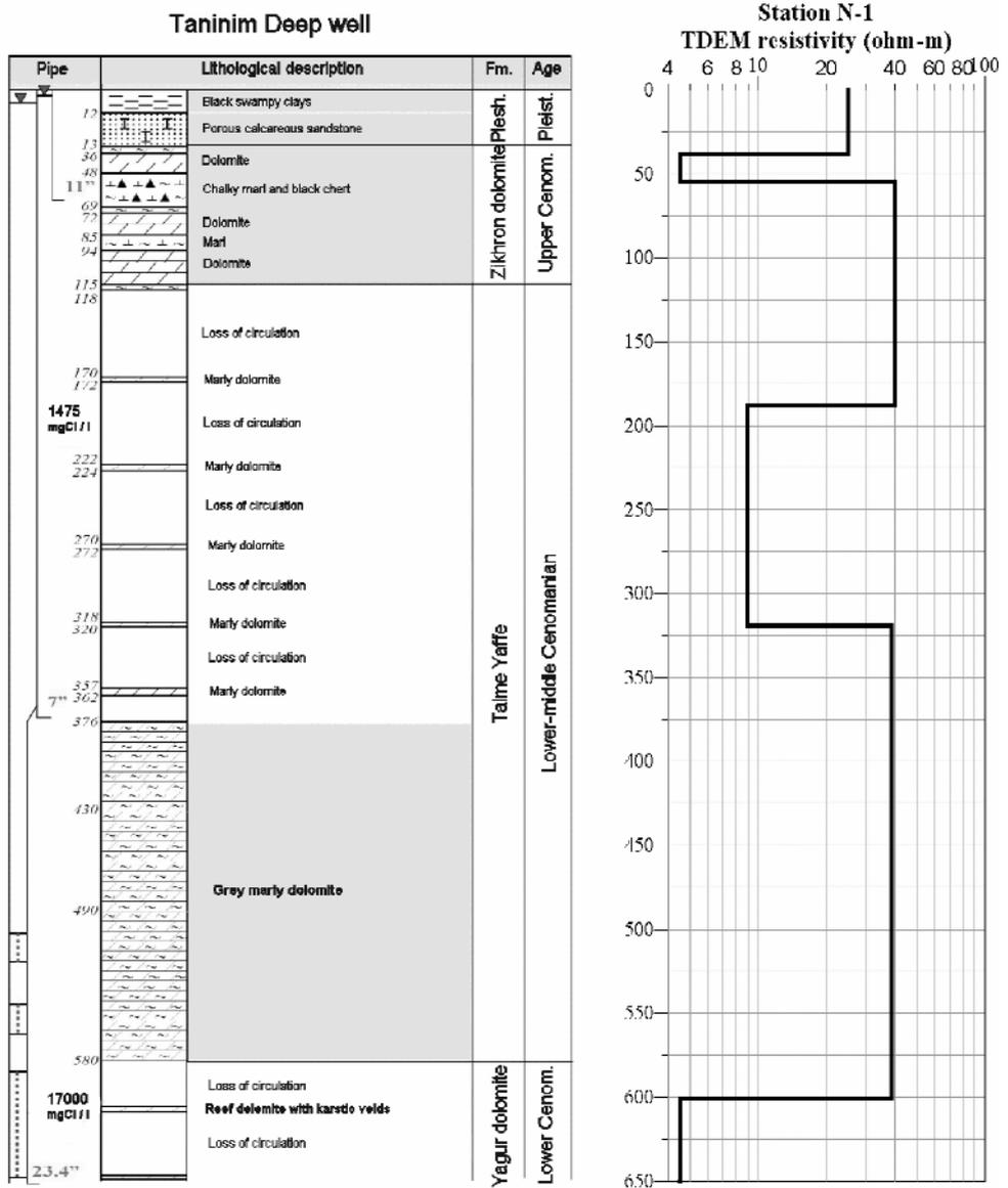
Figure 5. Comparison of TDEM results with borehole data from the Tanim Deep well. The low TDEM resistivities below 600 m depth are in agreement with the high groundwater salinity below the interface.
