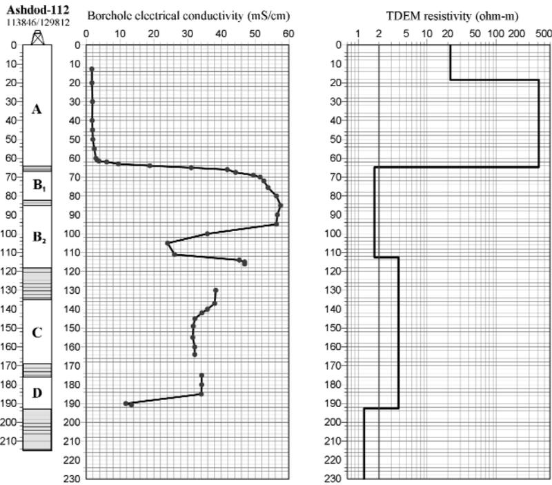
**Figure 2.** Comparison of the interpreted TDEM resistivity vs. depth model (in the right) with the borehole electrical conductivity profile (in the middle). The very left column shows the division of the aquifer into sub-aquifers A, B<sub>1</sub>, B<sub>2</sub>, C and D.
