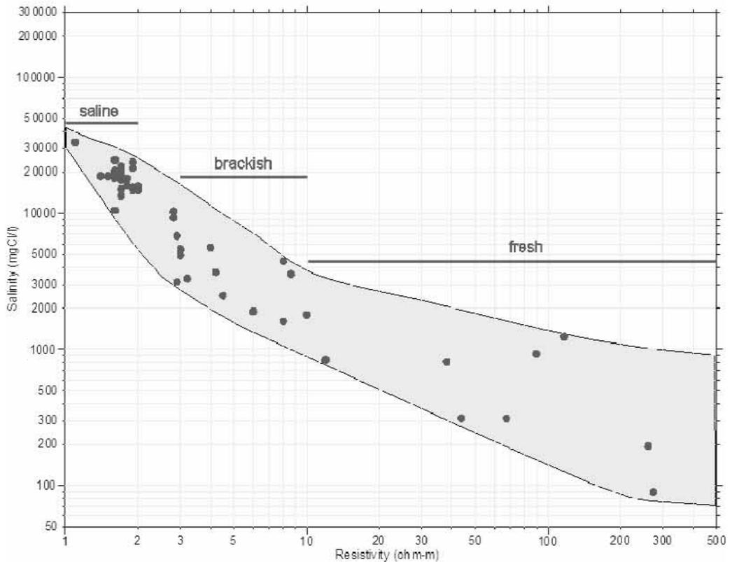
**Figure 3.** Resistivity-chlorinity calibration data based on 43 TDEM measurements carried out near observation wells along the Mediterranean coastal aquifer of Israel.
