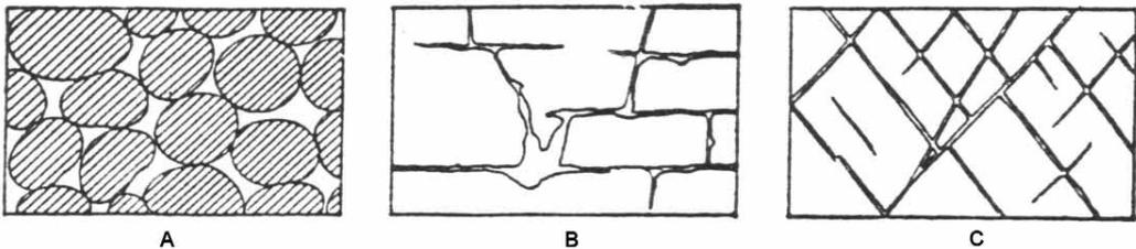
**Figure 6.** Diagram showing different types of rock interstices and the relation of rock texture to porosity. (A) Well-sorted sedimentary deposit having high porosity; (B) rock rendered porous by solution; (C) rock rendered porous by fracturing (after O.E. Meinzer, 1942).
