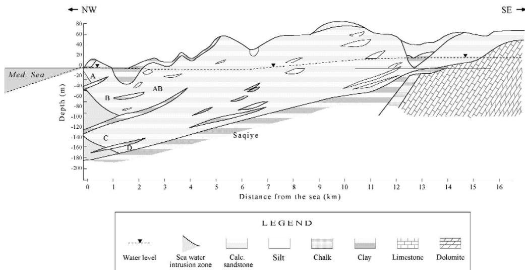
Figure 1. Typical hydrogeological cross-section of the Mediterranean coastal aquifer.
