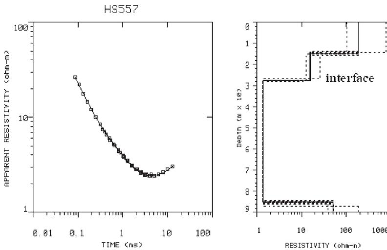
**Figure 4.** TDEM data collected at station HS557 in the Mediterranean coastal aquifer of Israel and the results of 1-D inversion including linear equivalence analysis by means of the TEMIX-XL interpretation software (Interpex, 1996).
