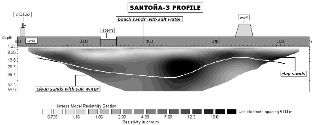
**Figure 5.** Image parallel to the coast, 5 m to the coastline, at San Martín beach (Santoña, Cantabria, N Spain). It shows the presence of an in-between level of slightly higher resistivity, which corresponds to a relatively less permeable sand with clay and, consequently, with a lower content of saline water due to their porosity being lower.
