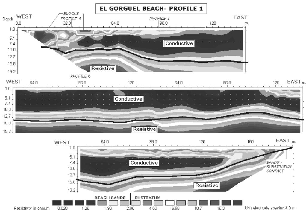
**Figure 2.** Electrical tomography parallel to the coast, close to the coastline on the El Gorguel. It is constituted by four continuous lines: line 1, to the left, lines 2+3, in the centre, and line 4, on the right.
