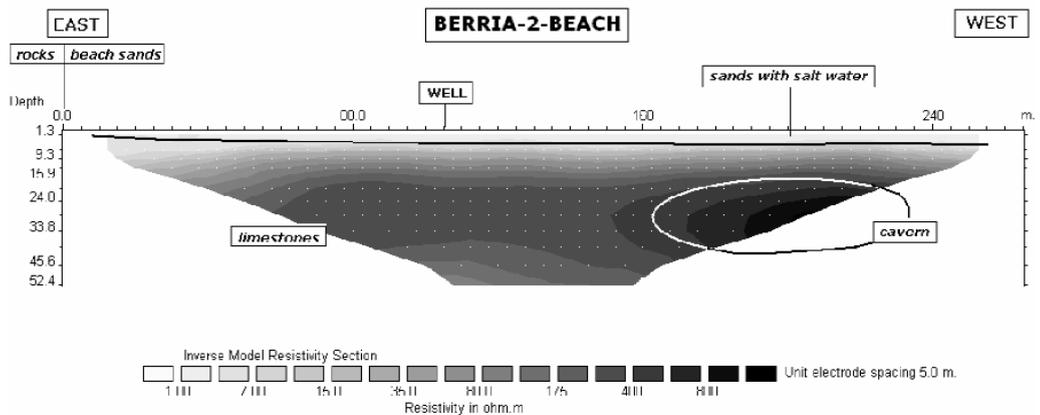
**Figure 6.** Image parallel to the coast, 20 m to the coastline, at Berria beach (Cantabria, N Spain). The presence of a layer with higher resistivity values and showing a cavity, which corresponds to relatively compact limestone formations, can be observed.
