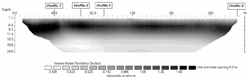
**Figure 4.** Image parallel to the coastline, 15 m to the coastline, at San Pedro del Pinatar (Murcia, SE Spain). It shows the presence of an interlayered unit of slightly higher resistivity, which corresponds to sand with a clay content that makes it less pervious and, consequently, with a lower proportion of saline water in their pores.
