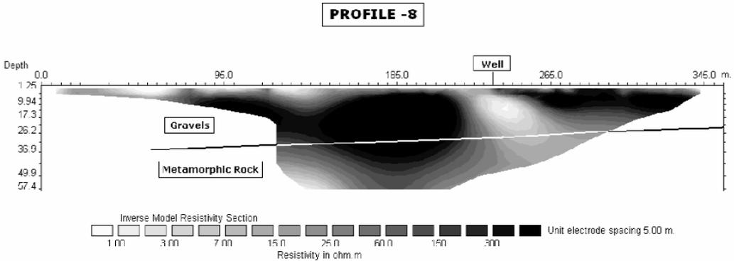
**Figure 3.** Image perpendicular to the coast showing a decrease in the resistivity sounding due to the presence of saline water.
