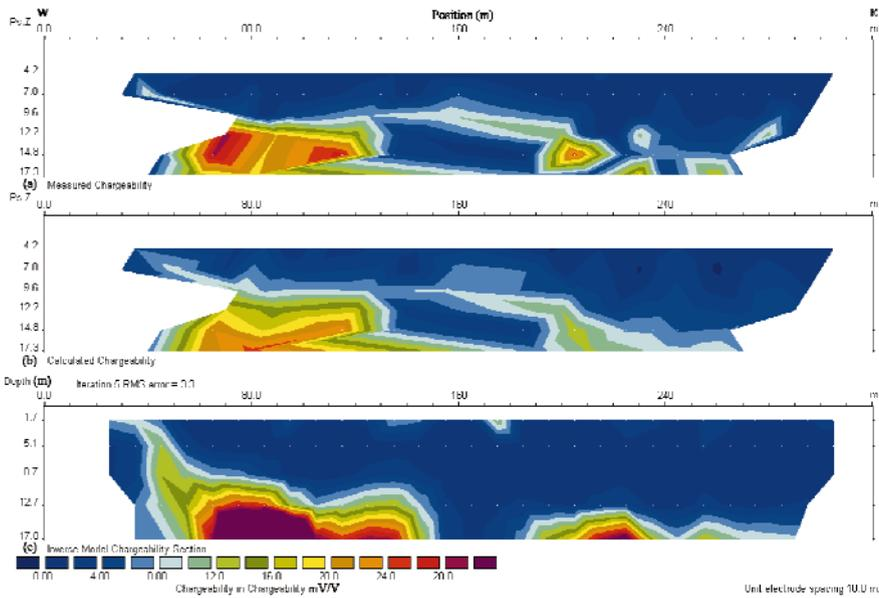
Figure 8. Chargeability pseudo-sections for survey line PC: (a) measured chargeability, (b) calculated chargeability, (c) inverse model chargeability.
