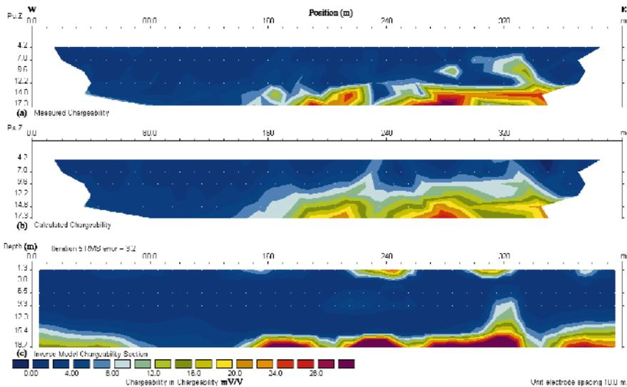
**Figure 5.** Chargeability pseudo-sections for survey line GA: (a) measured chargeability; (b) calculated chargeability; (c) inverse model chargeability.
