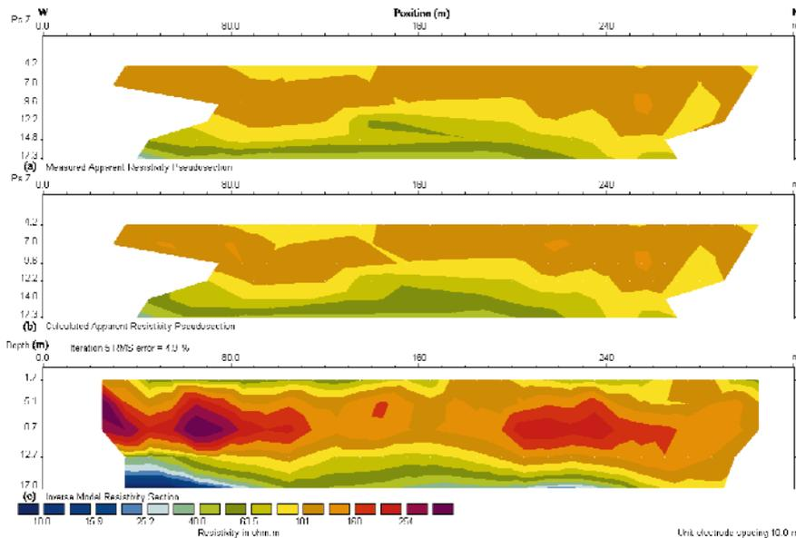
Figure 7. Apparent resistivity pseudo-sections for survey line PC: (a) measured apparent resistivity, (b) calculated apparent resistivity, (c) inverse model resistivity.
