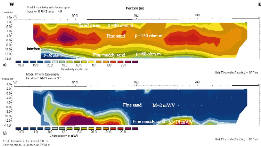
Figure 9. (a) Resistivity and (b) chargeability model sections for survey line PC interpreted in terms of local geology.
