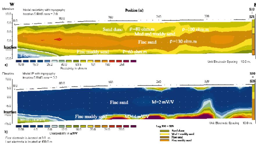
Figure 6. (a) Resistivity and (b) chargeability model sections for survey line GA interpreted in terms of local geology.
