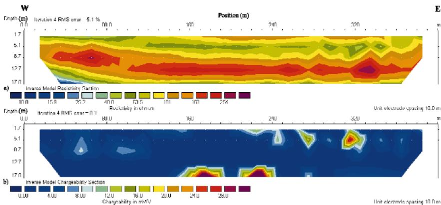
**Figure 2.** Modelling including negative IP values (line GA): (a) resistivity and (b) chargeability.
