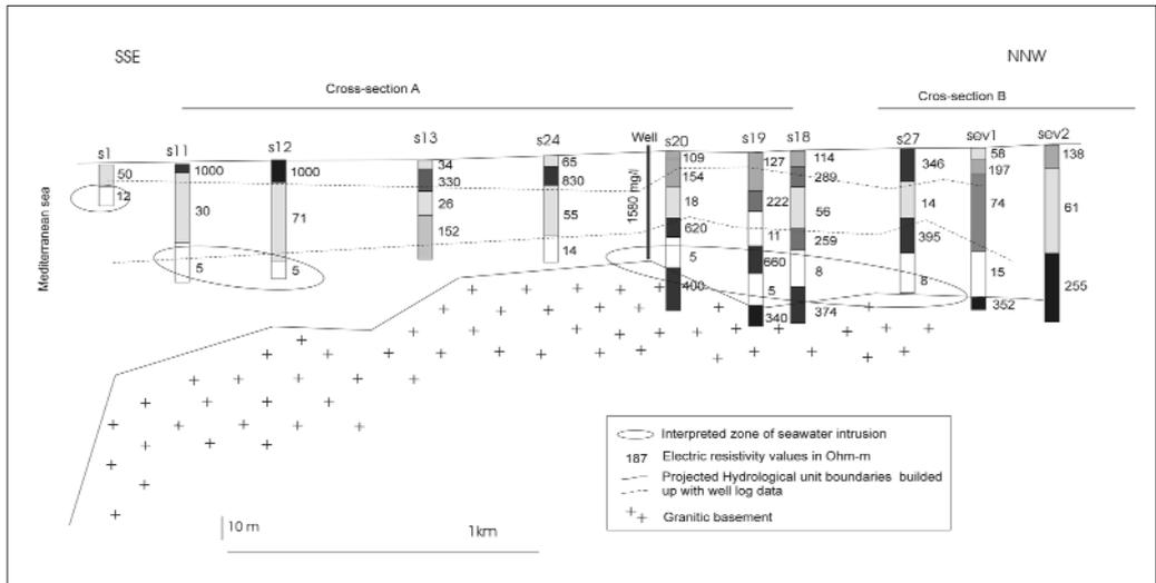
**Figure 7.** Geoelectrical cross-section along the riverbed obtained from VES data. Dashed lines are the projection of the aquifer unit boundaries after the well lithological logs. Chloride information (in mg/L) is from the ACA monitoring salinity network (February 2003). (VES location is in Figure 4, straight-lined along ERT sections).
