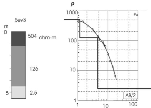
**Figure 5.** Typical VES near the coast. Note the high conductivity layer at the base of the model, associated to seawater.
