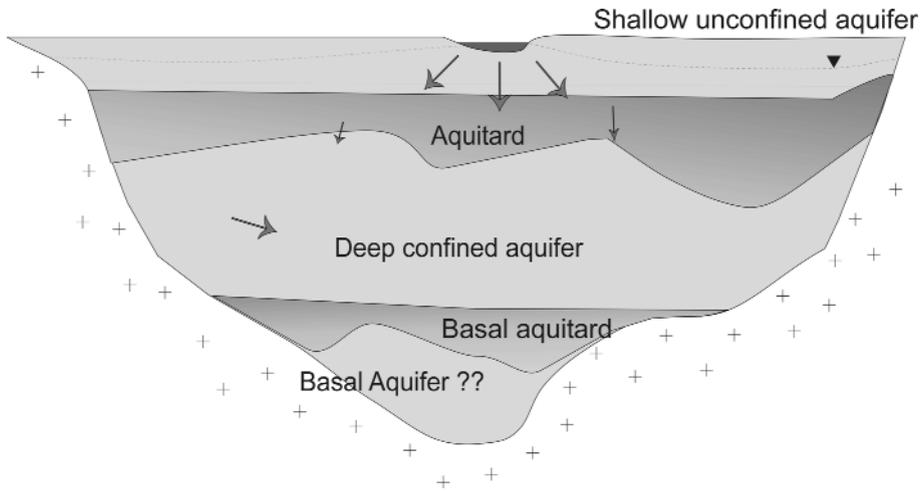
**Figure 3.** Hydrogeological model of the Baixà Tordera aquifer system.
