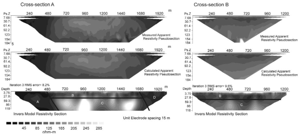
**Figure 8.** 2D geoelectrical cross-sections obtained from ERT. Top: measured apparent resistivity pseudo-section (PsZ: layer measured depth); middle: calculated apparent resistivity pseudo-section (model response); bottom: inverse model resistivity section. (See location in Figure 4).
