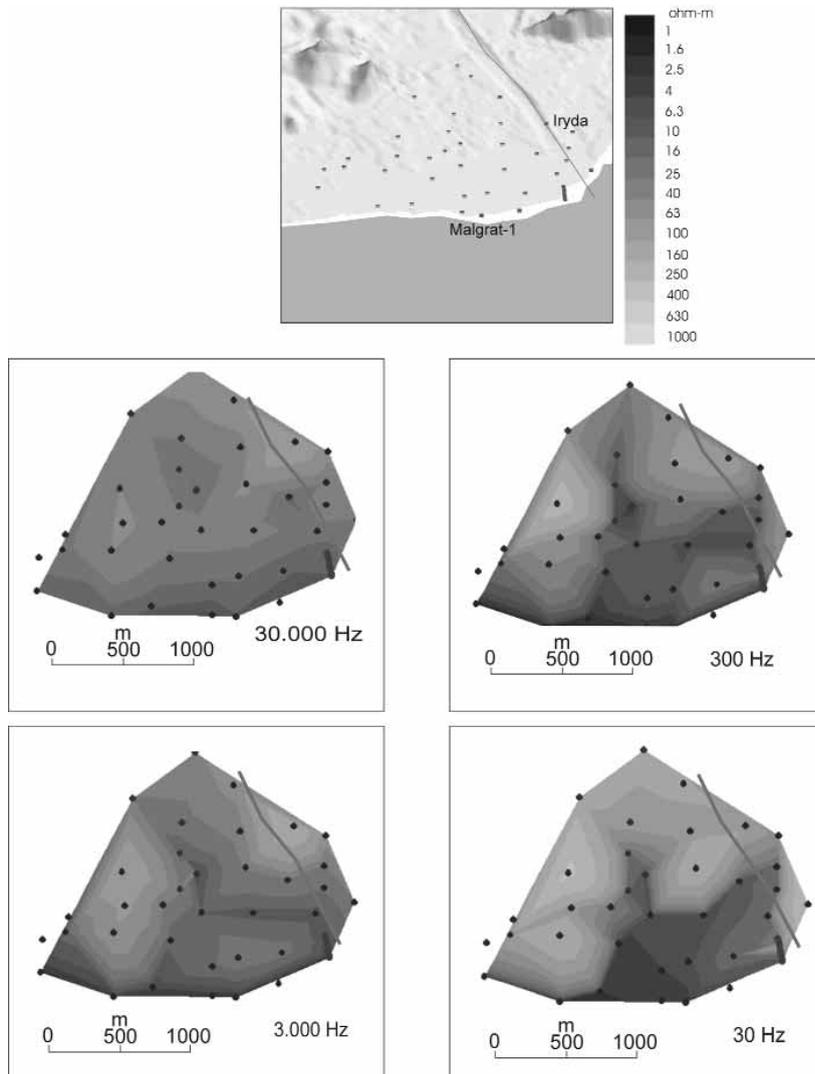
**Figure 9.** Apparent resistivity maps obtained from the phase determinant of the audiomagnetotelluric impedance tensor.
