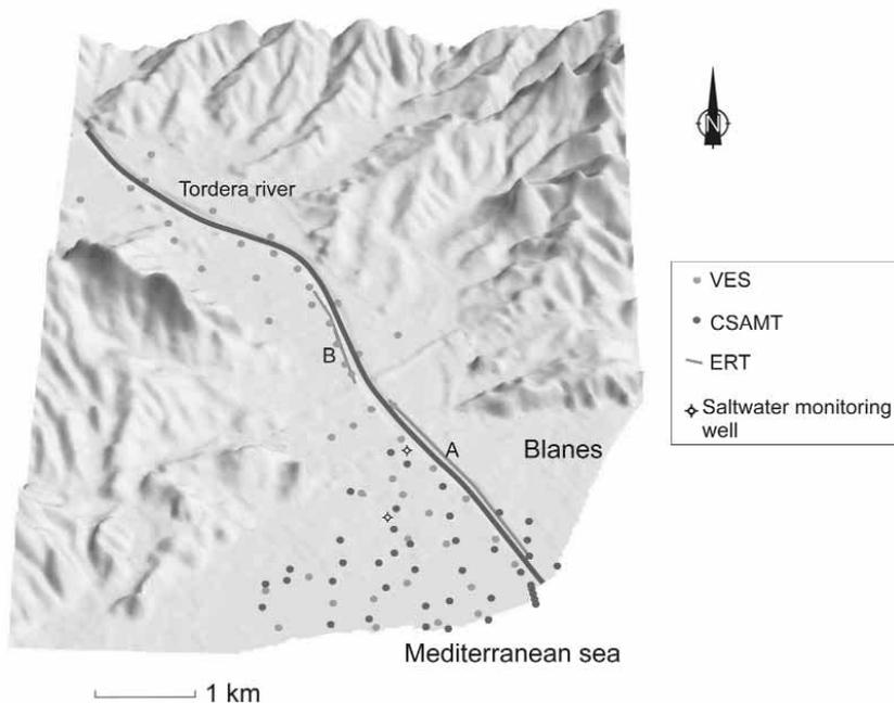
**Figure 4.** Site location of the geophysical and hydrochemical data. Lines: ERT profiles, light grey points: vertical electrical soundings (VES); dark grey points: control source for audiomagnetotelluric soundings.
