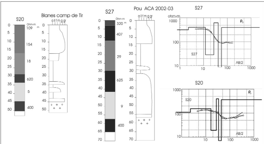
**Figure 6.** Interpretation of two VES (# 20 and 27) using lithological information. Right diagram:  $\rho_a$ -AB/2 ( $\rho_a$ =apparent resistivity; AB/2 distance between electrodes) data and interpreted resistivity layer model. Lithology log and interpreted electrical resistivity layer model: note the presence of a conductive structure (a gravel layer) on top of the basement; it has been interpreted as seawater contaminated zone.
