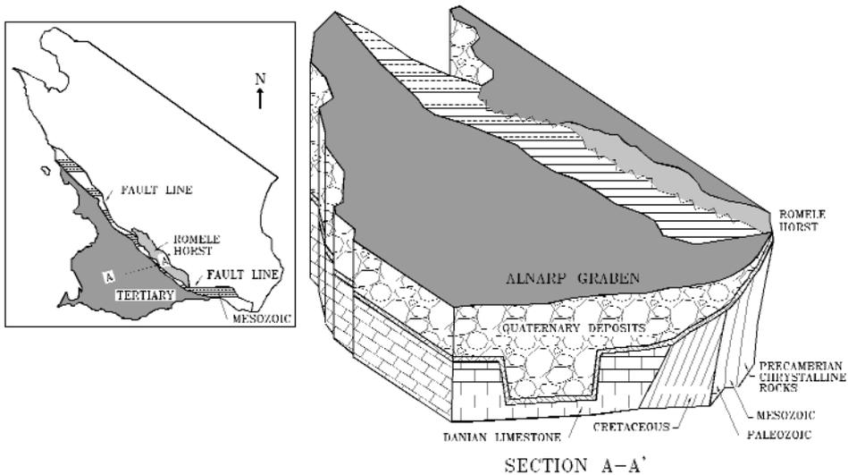
**Figure 3.** Cross section A-A' shows Quaternary deposits and bedrock from southwest to northeast in southwest Scania. The northeastern section ends at the Romele horst, an area where uplift occurs due to tectonic activity. From Fredén (1994).
