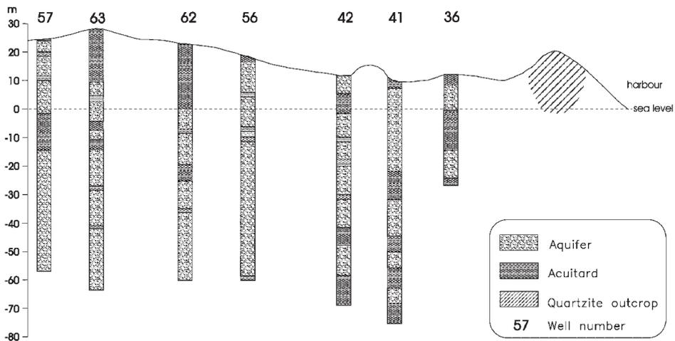
**Figure 2.** Schematic geological profile of the harbour graben.
