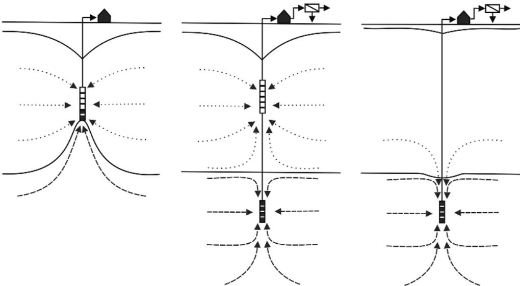
**Figure 1.** Schematic presentation of a salinizing well, the fresh-holder and a brackish well.
