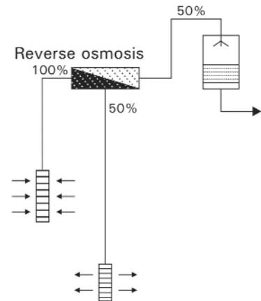
**Figure 2.** The pretreatment of the brackish groundwater with membranes
