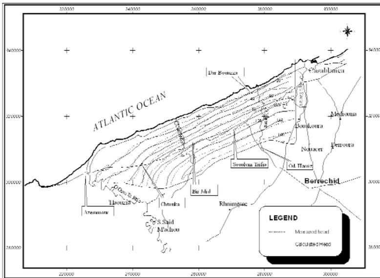
**Figure 4.** Calibrated and observed groundwater levels for the year 1949.
