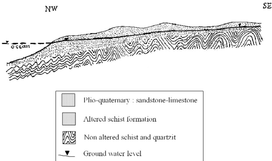
Figure 2. Schematic hydrogeological cross section of the Chaouia aquifer.
