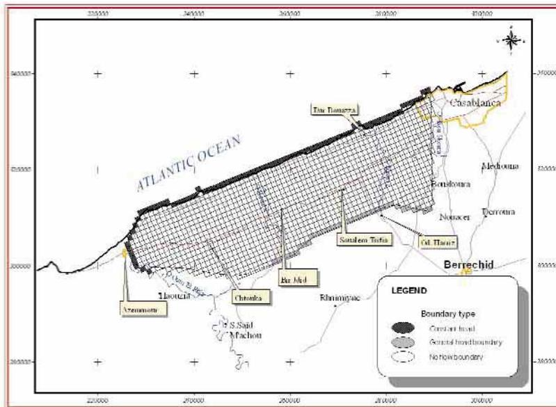
Figure 3. Finite-difference grid and boundary conditions for the Chaouia regional model.
