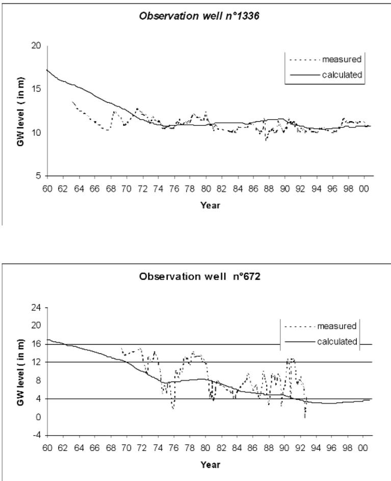
**Figure 5.** Calibrated and observed water level evolution.
