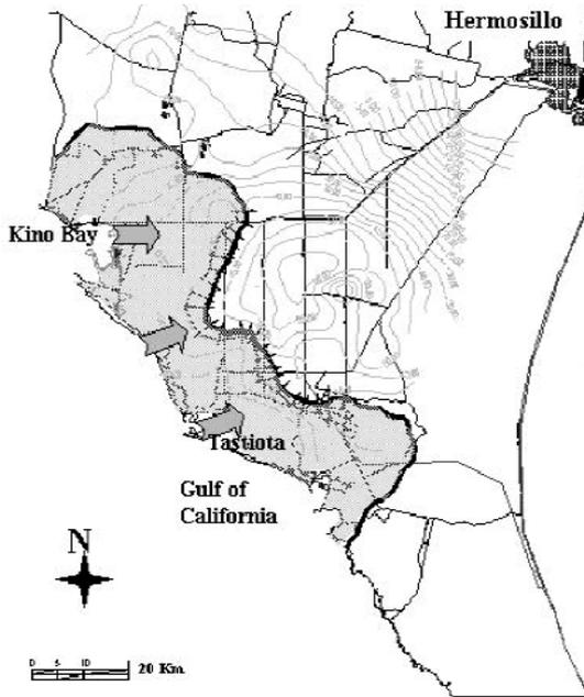
**Figure 6.** Groundwater surface level in the Costa de Hermosillo aquifer in 1999, gray arrows show the three seawater flow paths.
