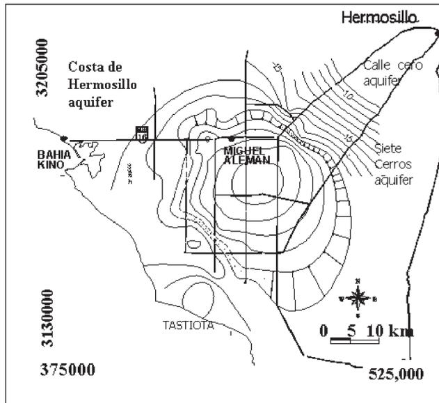
**Figure 5.** Monitoring wells and groundwater surface level in 2003.
