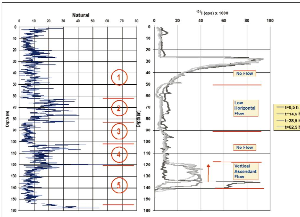
**Figure 6.** - Natural gamma log and results of a flow-test with  $^{131}\text{I}$  (single-well technique) conducted in La Herriza borehole.
