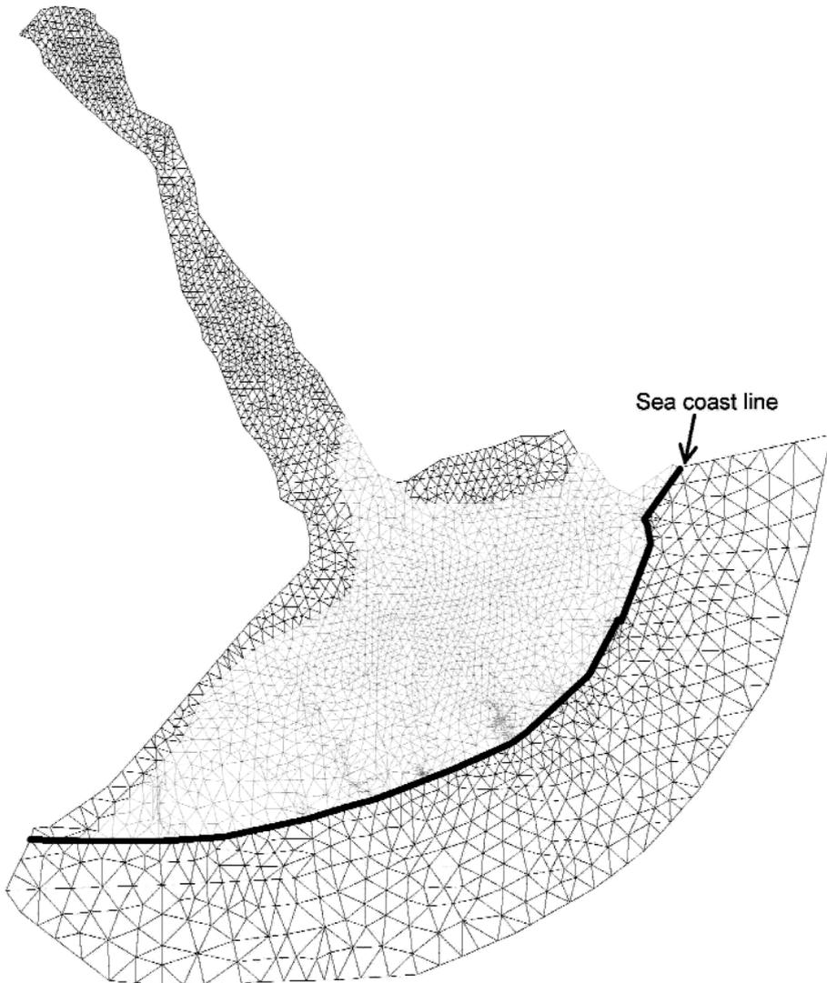
**Figure 4.** Finite element mesh divided into two layers (grey and black) connected by 1D elements. The complete mesh is composed of 4411 nodes and 9848 elements.
