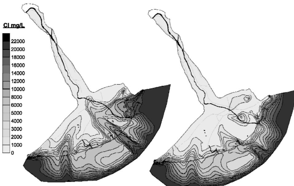
**Figure 8.** Left: simulation of the future evolution of salinity in the main aquifer of the delta (year 2037) if the pumping wells move inland as a consequence of salinity making the pumped water undrinkable. Right: Hypothetical situation in year 2037 if the current situation is remediated with some additional measures such as an injection barrier and recharge ponds.
