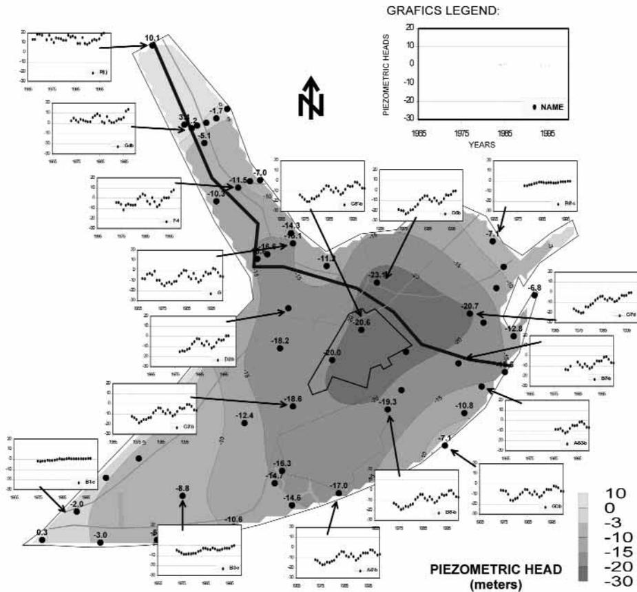
**Figure 1.** Piezometric surface corresponding to the Main Aquifer in 1976, year of maximum depression. Hydrographs in several points of the aquifer show the complex evolution of the hydraulic heads.
