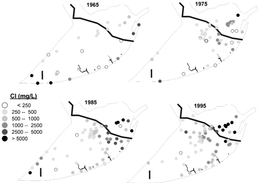
**Figure 2.** Chloride concentration data evolution in the main aquifer of the Llobregat delta. Two fingers of high salinity can be observed advancing towards the main pumping fields in the center of the Llobregat delta.
