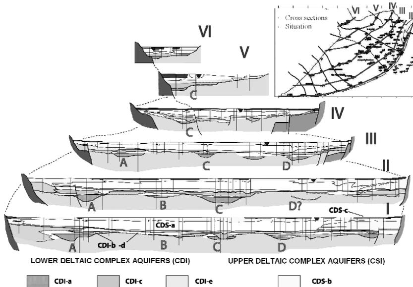
**Figure 3b.** Conceptual model of the incised systems of the called Lower Detritic Complex. Gravels and conglomerates represent the different incised systems. Between the coarse sediments there are silts and sands are found. The lower grey area represents the Pliocene Blue Marls, and the dark-grey the Miocene and pre-Miocene basement.
