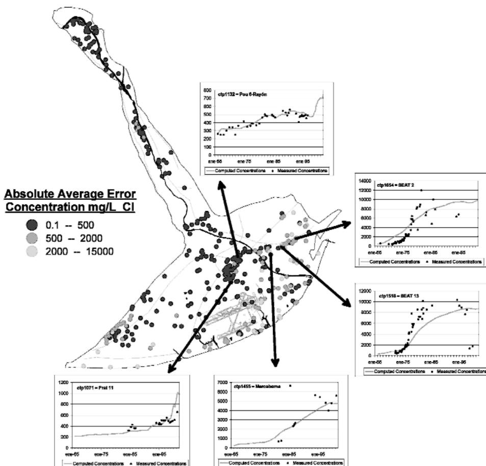
**Figure 6b.** Chloride calibration errors in the main aquifer, defined as the mean difference between the calculated and the measured concentration data at any given observation location. The dark dots represent wells whose mean difference is less than 500 mg/L of chloride. The time evolution of calculated and measured concentration in several wells is also shown.
