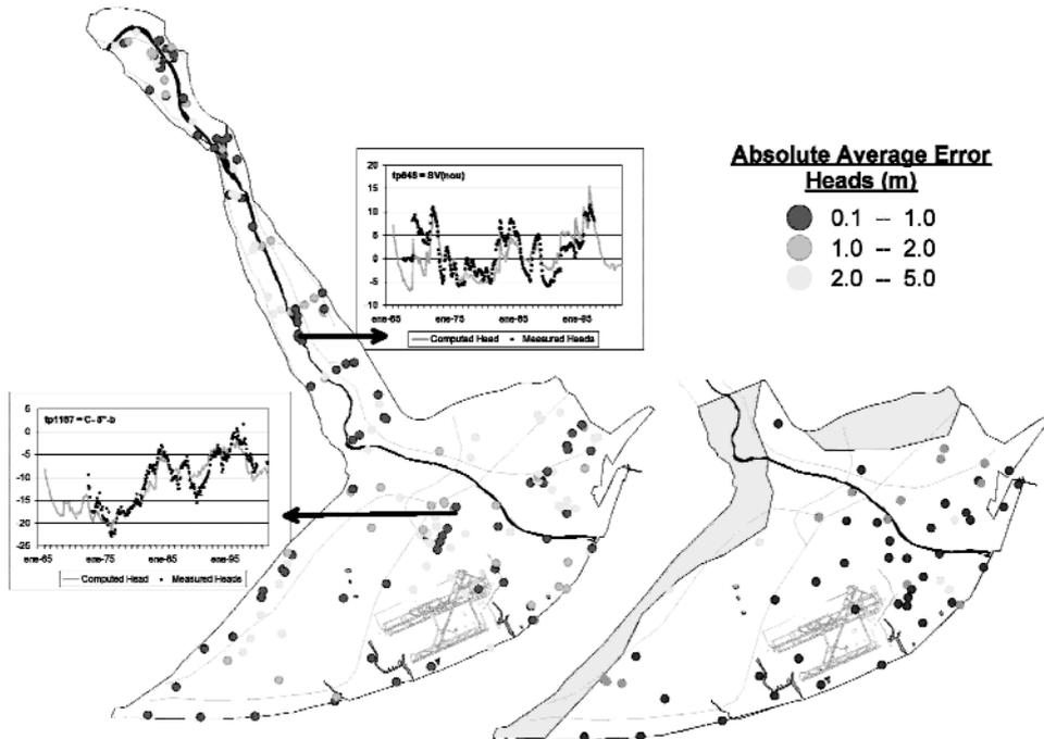
**Figure 6a.** Head calibration errors, defined as the mean difference between the calculated and the measured head data at a given observation point. The dark dots represent wells whose mean difference is less than a meter. The time evolution of calculated and measured heads in two wells is also shown. The main aquifer is displayed on the left, while the upper aquifer is on the right.
