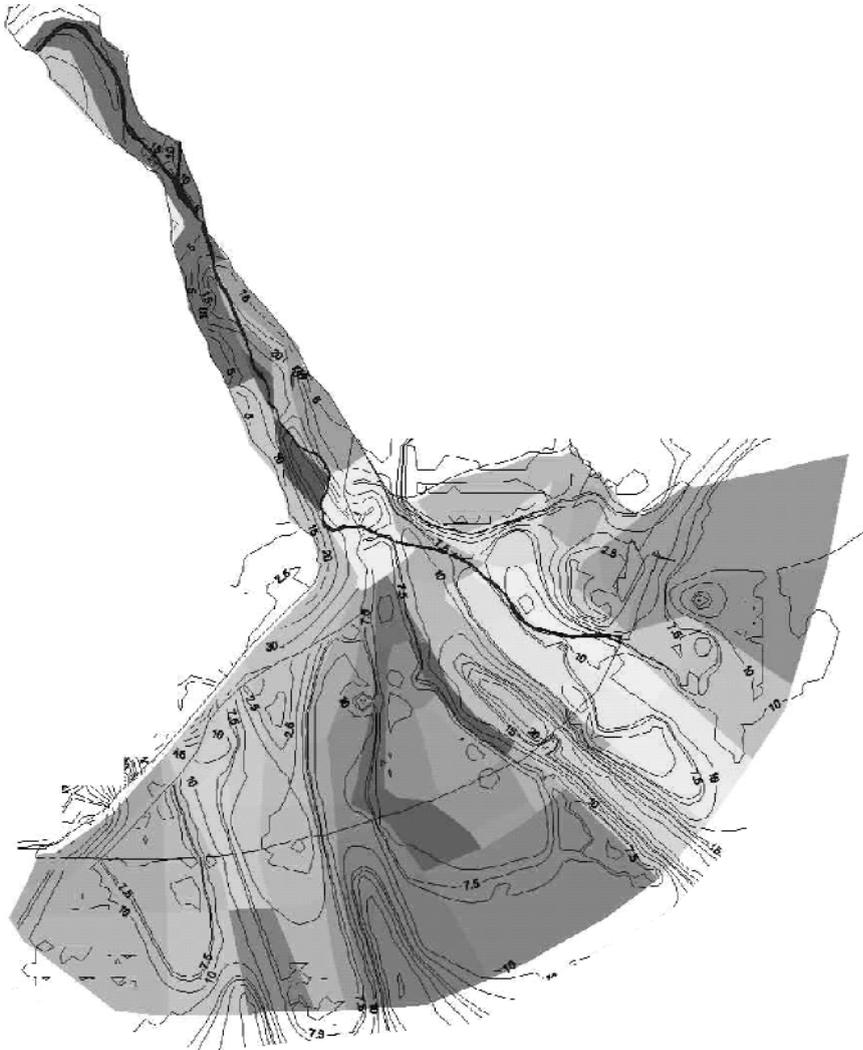
**Figure 5.** Map of transmissivity zones. 101 constant transmissivity zones are defined, based on several criteria: aquifer thickness, lithofacies, hydraulic tests and sediments grain size distribution of the sediments. Aquifer thickness isolines (in meters) are plotted over the map.
