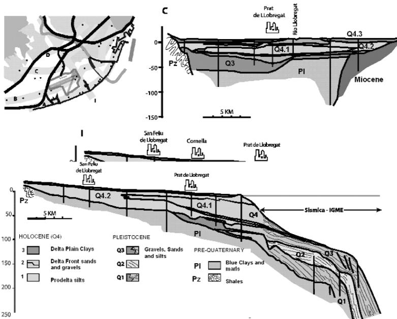
**Figure 3a.** Geological cross-section of the emerged and submerged delta based on old MOP data and from a reflexion seismic survey performed by IGME. Vertical scale in meters. The silt wedge separates the upper and main (lower) aquifers. Other old Quaternary deltas (Q1-Q3) are part of a hydrologically unknown lower aquifer system. The modern delta (Q4) was formed about 18000 years ago, although its progradation took place during the last 6000 years.
