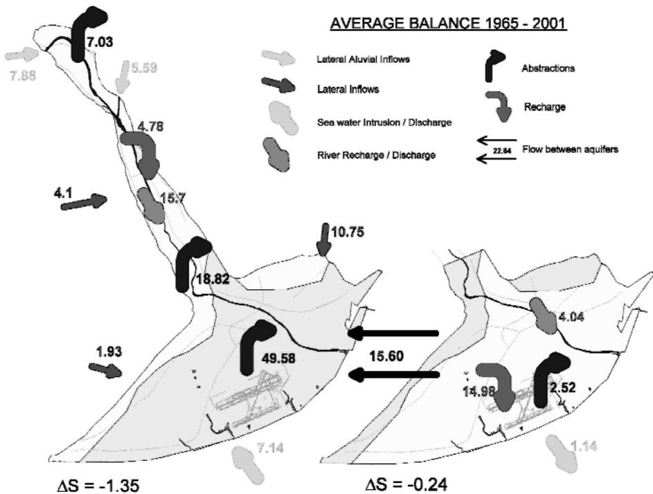
**Figure 7.** Water mass balance scheme for the Llobregat delta aquifers expressed in  $Mm^3/y$ . The mass balance for the main aquifer is shown on the left side and for the upper aquifer on the right. The black arrows show the flux from the upper to the main aquifer.
