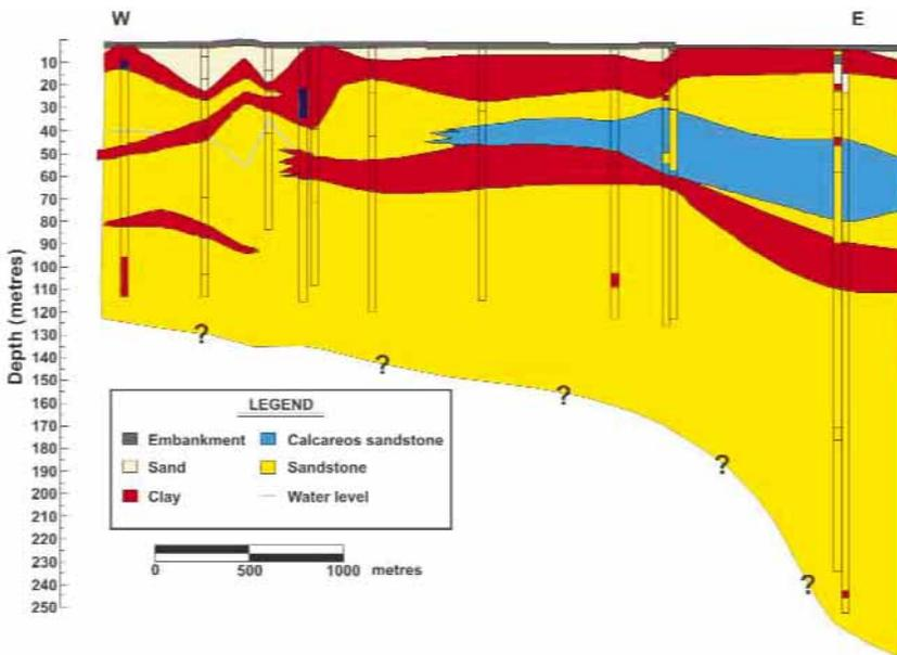
**Figure 2.** West / East cross-section, with the Boa Viagem (upper) and Beberibe (lower) aquifers.
