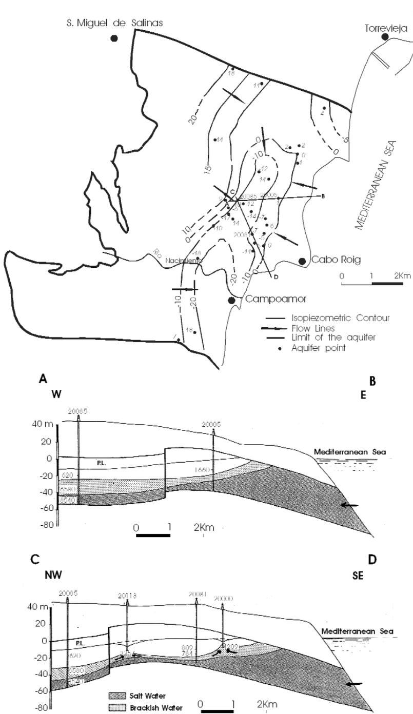
Figure 5. Marine intrusion in the Cape Roig aquifer.
