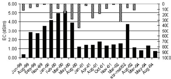
Figure 7. Electrical conductivity of groundwater influenced by rainfall.
