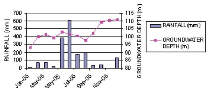
Figure 4- Rainfall and groundwater potentiometric depth in 2005 in Boa Viagem Beach.
