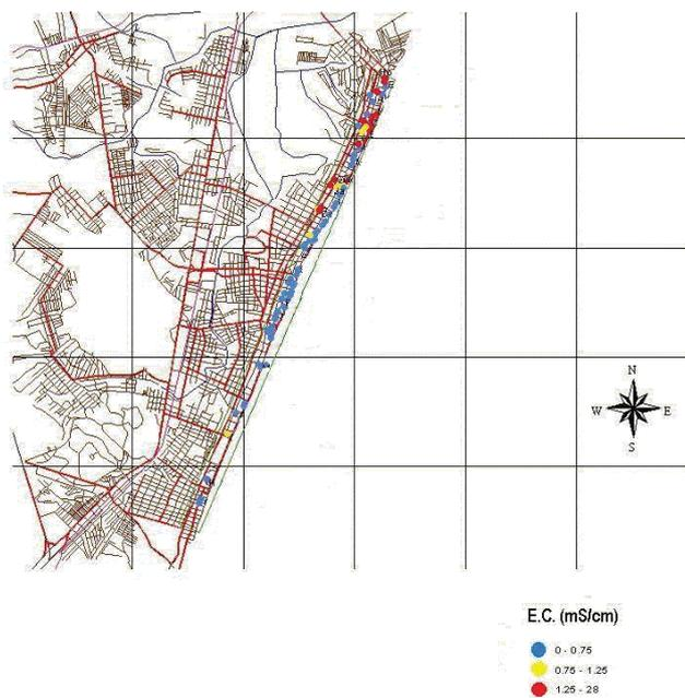
Figure 8- Electrical conductivity mean values in Boa Viagem coastal zone.
