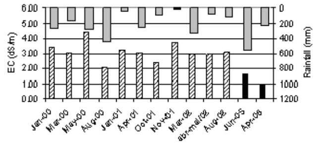
Figure 10- Electrical conductivity levels in two nearby wells, in the same building.
