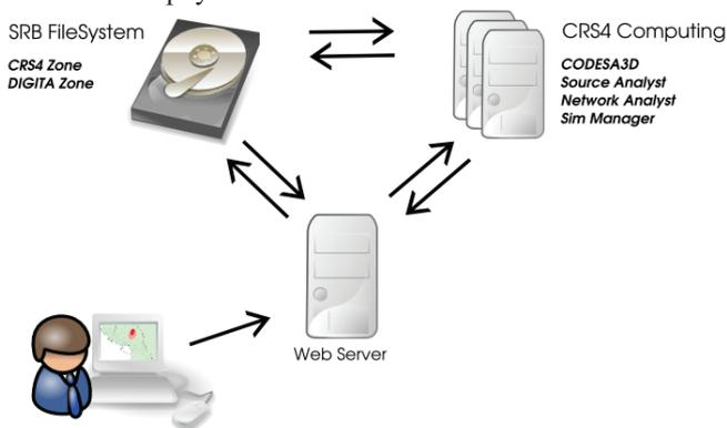
Figure 2. Logical organization of data flows. Users access only the front end, through which computing resources and data are accessed.
