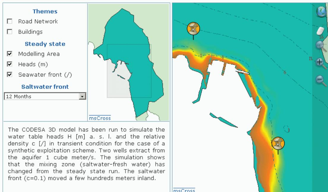
Figure 4. This module produce a real time geo-raster showing the salt water intrusion by means of the open source GRASS module. The effect of pumping is spatially dependent.
