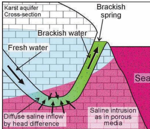
Figure 2: Conceptual cross section of a coastal karst aquifer with a diffuse saline intrusion
