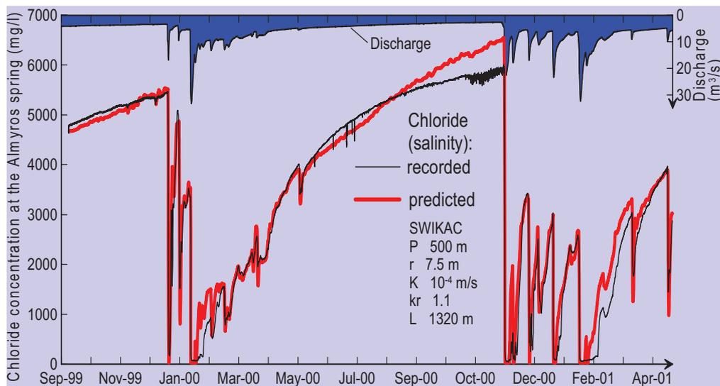
Figure 7: Recorded chloride concentration and that predicted with the SWIKAC model at the Almyros of Heraklio spring (Crete) (Arfib 2001)
