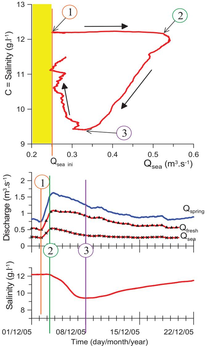
Figure 6: Hysteresis curve  $Q_{sea}$ - $C$  of a high water event from 01 December to 22 December 2005 at the Port-Miou spring, and evolution with time of the total discharge ( $Q_{spring}$ ), discharge of seawater ( $Q_{sea}$ ), discharge of freshwater ( $Q_{fresh}$ ) and salinity. [modified from Arfib et al. 2006]
