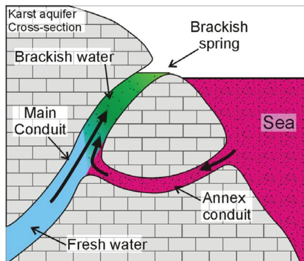
Figure 1: Conceptual cross section of a coastal karst aquifer with a connection of conduits to the sea.
