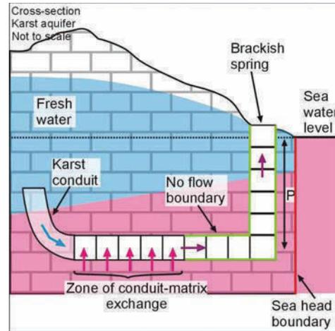
Figure 3: Conceptual model of the numerical SWIKAC model
