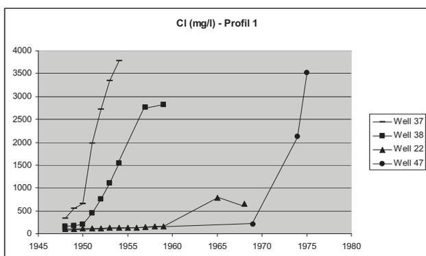
Fig. 3 Evolution of chloride concentration in two profiles perpendicular to the coast line
