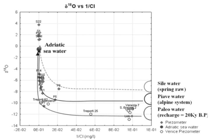
Fig. 11. The relationship between chloride and oxygen isotopes (1/Cl vs δ<sup>18</sup>O) highlights the mixing and dilution trend of water in the northern sector of the Venice Lagoon territory: three different mixing lines related respectively to the Sile water (spring raw) with fresh continental water values, the Piave river, a
