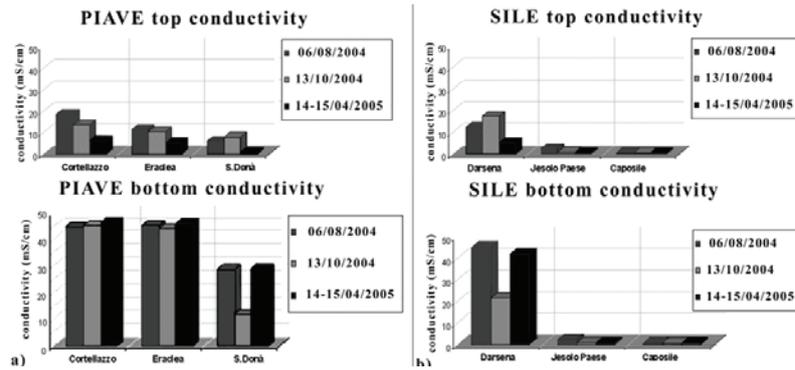
Fig. 5. EC measurements along the Piave (a) and Sile (b) rivers highlight the different behaviours of the two water courses: a salt water wedge can be found on the Piave riverbed for about 20 km, aided by the presence, at Eraclea, of a topographic depression, whereas in the Sile river, the contamination is effectively diminished with fresh water dispersion from the system of springs
