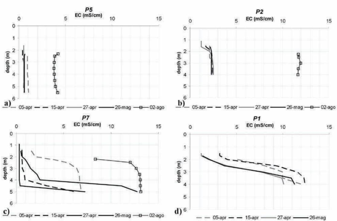
Fig. 2. Conductivity logs showing the electrical conductivity trend for wells characterized by low salinity (P5) and high EC values ranging from 3,5 to 12,8 mS/cm (P2-P7-P1)
