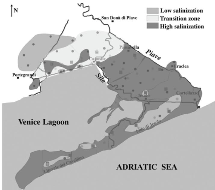
Fig. 7. Map of the superficial salinization of the northern sector of the Venice lagoon mainland obtained by a combination of EC Logs data and VES soundings
