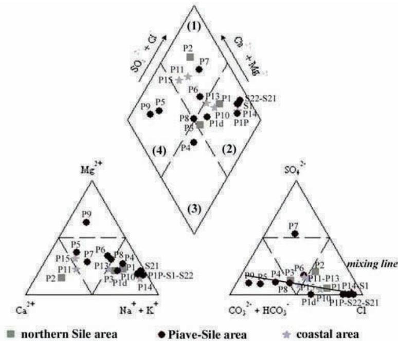
Fig. 8. The chemical hydrofacies for the samples collected from the unconfined aquifers: generally it is possible to recognize a progressive enrichment in Cl content near the Piave river, in connection with an old lagoon channel and paleochannel, as well as in the coastal zone away from sand dunes, where the effects of fresh water lenses is not able to contrast the salinization effects
