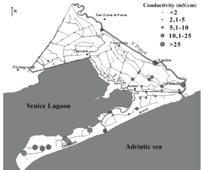
Fig. 3. Conductivity values (EC logs) of the superficial hydrography (rivers and channels) in order to determine the utility of using their water to irrigate the land. This also allow for the determination of increasing
