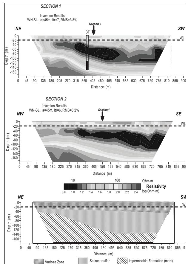
Fig. 13. Electrical Resistivity Tomography sections and subsequent interpretation.
