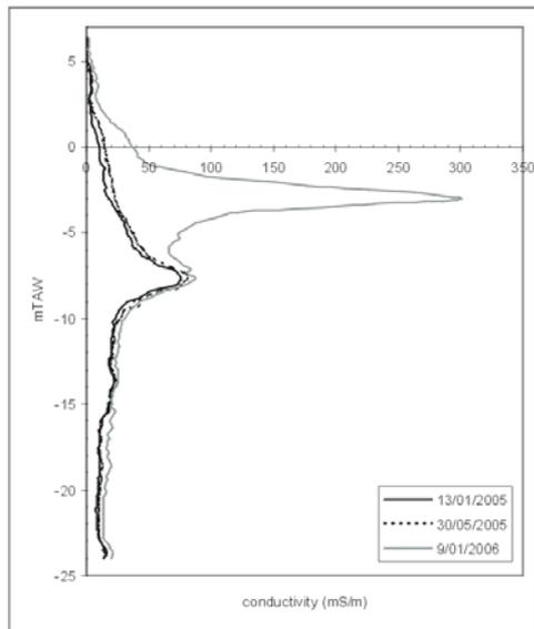
Fig. 9. Electrical conductivity measured in P8.
