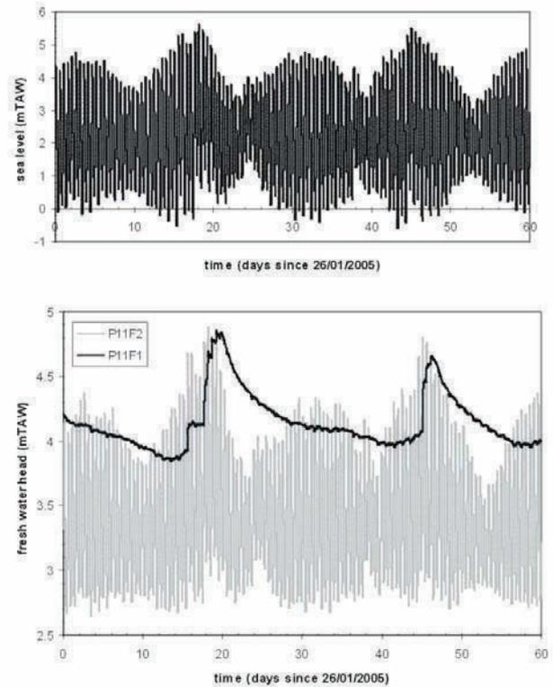
Fig. 10. Sea level fluctuations and fresh water heads in P11F1 and P11F2 from 26/01/2005 onwards.
