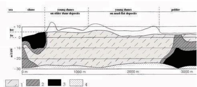
Fig. 4. Distribution of fresh (1), brackish (2) and saline (3) water in the dunes of the Westhoek Nature Reserve. A clay layer (4) forms the lower boundary of the aquifer.
