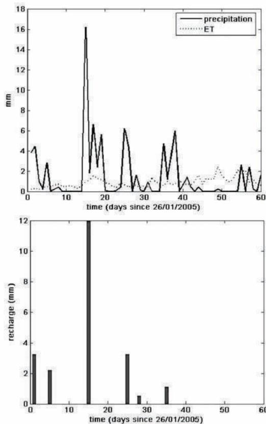
Fig. 11. Daily precipitation, evapotranspiration (ET) and recharge from 26/01/2005 onwards.
