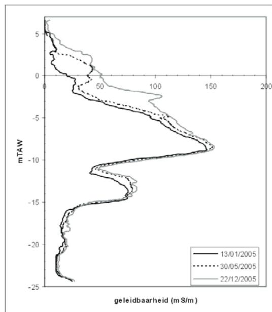
Fig. 8. Electrical conductivity measured in P6.
