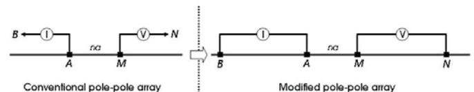
Fig. 3 Schematic comparison diagram of surface electrical resistivity survey between conventional and modified pole-pole array.
