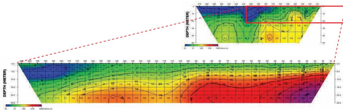
Fig. 7 2-D inversion results showing the boundary between seawater wedge and relatively fresh bedrock
