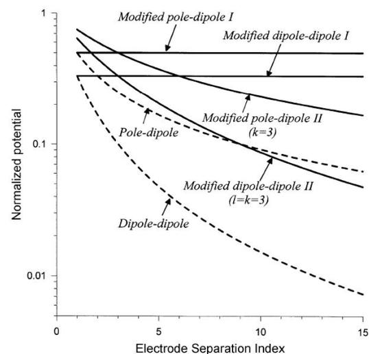
Fig. 4 Normalized potential variations of modified electrode arrays in the homogeneous half-space. (Kim et al., 2001).
