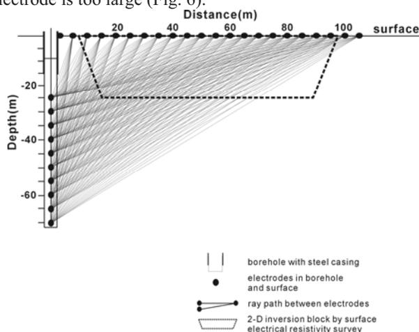
Fig. 6 Ray path of electrical resistivity tomography using single well and 2-D inversion block by surface electrical resistivity survey
