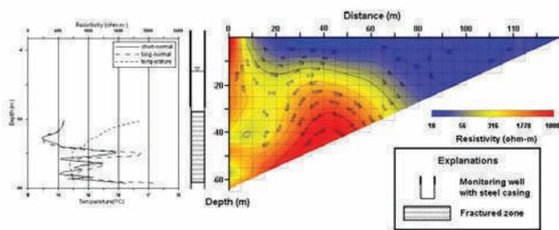
Fig. 9 Joint inversion result of electrical resistivity tomography using single well and surface resistivity survey compared to electrical resistivity logging.
