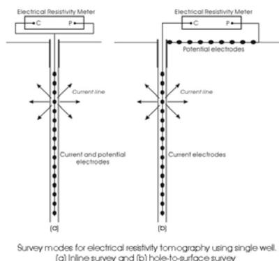
Fig. 5 Survey modes for electrical resistivity tomography using single well.
