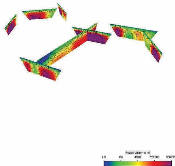
Fig. 8 3-D fence diagram of resistivity shows the boundary between seawater wedge and relatively fresh bedrock in a small watershed.
