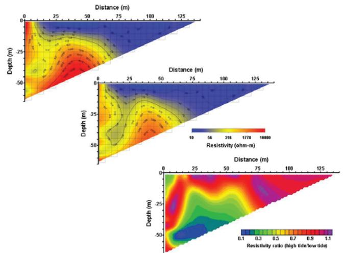
Fig. 10 Ratio of resistivity variations between high tide and low tide.
