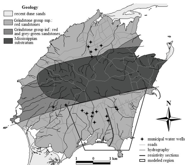
Fig. 2. Geological map of Grindstone Island with location of modelled region and layout of the selected resistivity profile correlated with modeling (Fig. 8).
