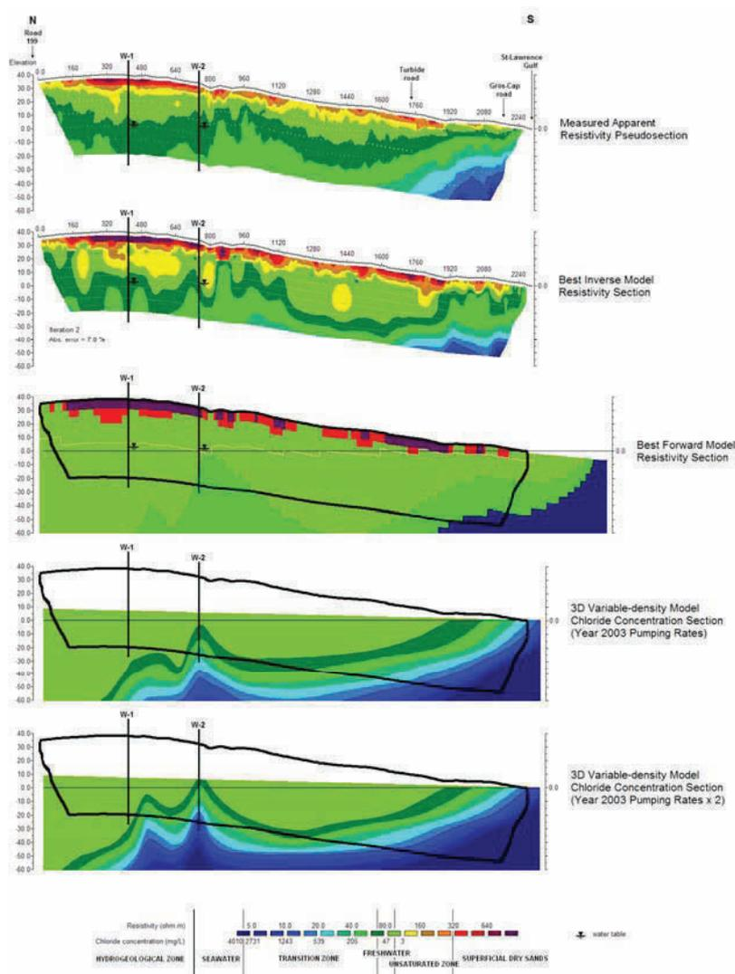
Fig. 8. Comparison between geophysical sections (3 Fig. on top, resistivity in ohm.m) and variable-density flow model sections (2 Fig. on bottom, chloride concentration in mg/L) of saltwater intrusion in the centre of modelled region (wells W-1 and W-2).
