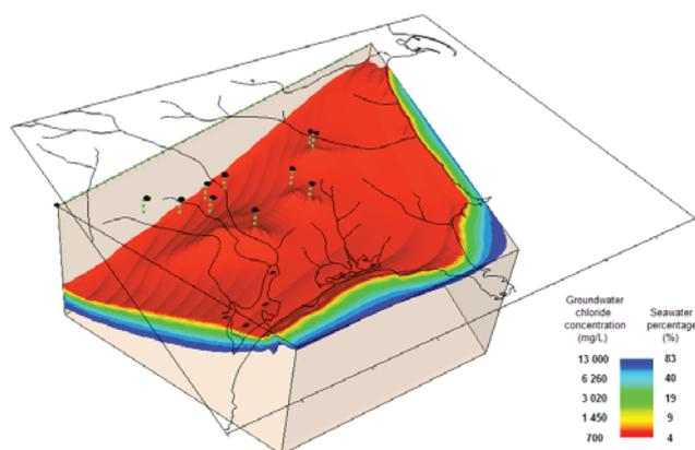
Fig. 5. 3D simulation of the freshwater/saltwater transition zone and saltwater intrusion spots in modelled region of Grindstone Island (vertical exaggeration is three times).
