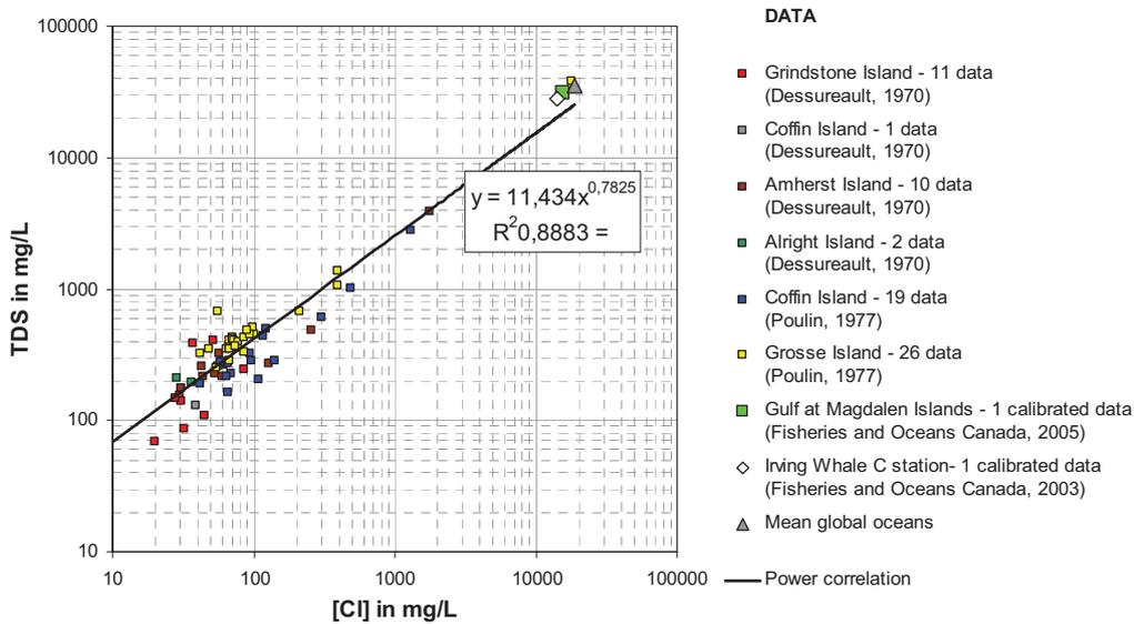
Fig. 7. Correlation between chloride concentrations and total dissolved solids (TDS) in Magdalen Islands' groundwater and seawater
