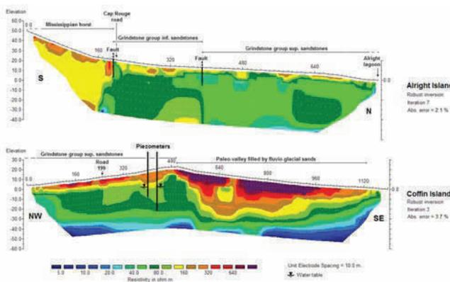
Fig. 3. Two typical inverse model resistivity profiles of Magdalen Islands
