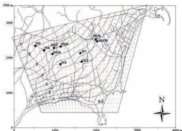
Fig. 4. Year 2003 simulated water table elevation (blue contour lines, in m above sea level) and velocity vectors (projected to horizontal) at 2.5 m under sea level
