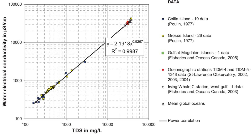
Fig. 6. Correlation between total dissolved solids (TDS) and electrical conductivity in Magdalen Islands' groundwater and seawater.
