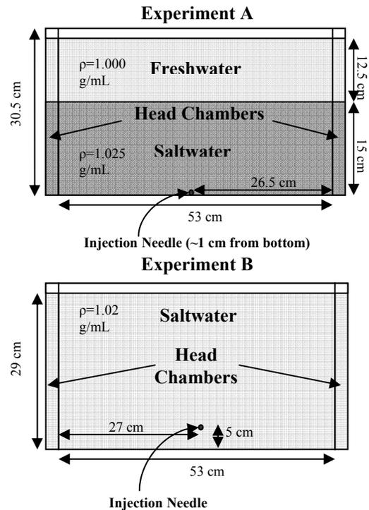
**Figure 1 (A and B). Physical model set-up for experiments A and B**
