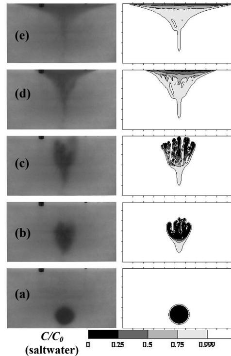
Figure 3. Experiment B and SEAWAT results: [times are from end of injection (sec)] (a) 27, (b) 369, (c) 685, (d) 1385, (e) 2631
