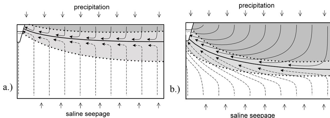
**Figure 1. Flow lines of infiltrating fresh water (grey) and upward seeping saline water (white), from the ditch to the middle of a field. a.) during initial lens formation and b.) at steady state (right). Solid lines: imaginary sharp interface. Dotted lines: observed mixing zone**
