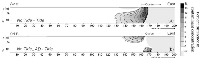
Figure 4. Percent difference in contaminant concentration with (a) constant dispersivity and (b) apparent dispersivity.
