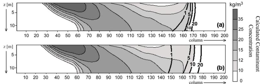
**Figure 1. Overlap of calculated contaminant concentration on freshwater/saltwater interface in simulation: (a) without tides, *NO TIDE*, and (b) with tidal variations, *TIDE*. Dark black contours represent salinity isosurfaces in  $\text{kg/m}^3$ .**
