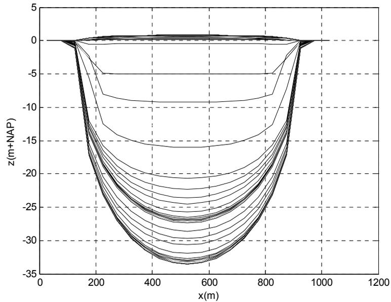
**Figure 1. Phreatic groundwaterlevel and position of the interface.**
