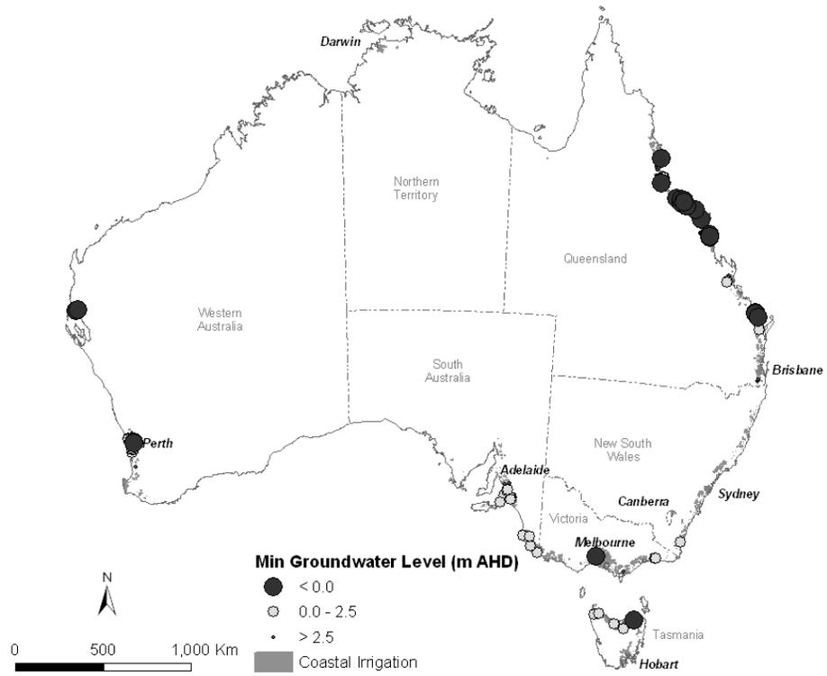
**Figure 8. Minimum (lowest) groundwater levels during the period 2000-2008**
