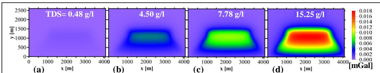
Abb. 3: Sensitivity of vertical gravity anomalies ( $\Delta g_z$ ) resulting from brine leakage of varying salinities (TDS). Applied TDS intrusion (a) is undetectable by modern micro-gravimeters (3-5  $\mu\text{Gal}$  precision) and the detectability starts for TDS  $\geq 4.5$  g/l (b-d).
