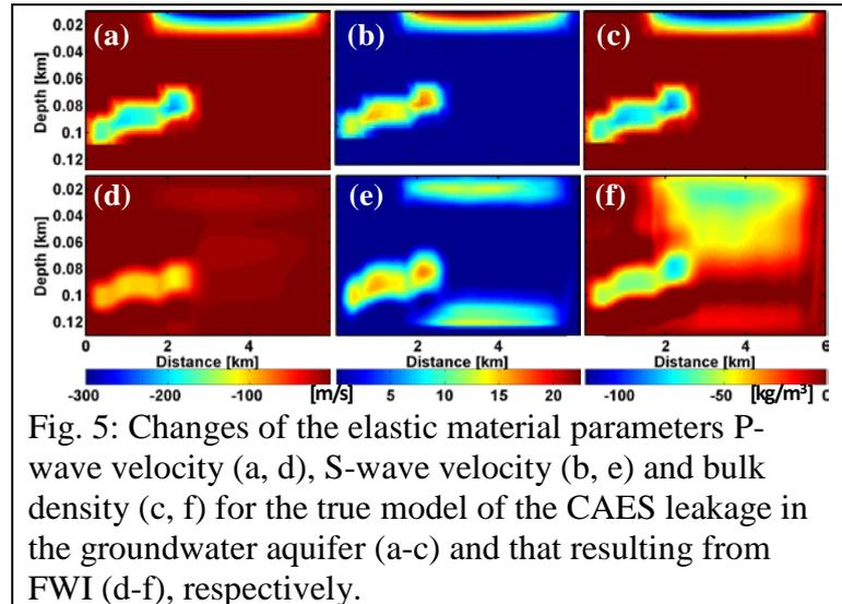
Fig. 5: Changes of the elastic material parameters P-wave velocity (a, d), S-wave velocity (b, e) and bulk density (c, f) for the true model of the CAES leakage in the groundwater aquifer (a-c) and that resulting from FWI (d-f), respectively.
