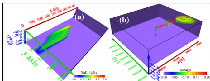
Figure 1: 3D saltwater and CAES leakages into shallow groundwater. After 10 years of leakage the density change of water is up to 4 kg/m<sup>3</sup> for saltwater intrusion (salinity 4 g/l, a) and -340 kg/m<sup>3</sup> for CAES (saturation 0.654, b).
