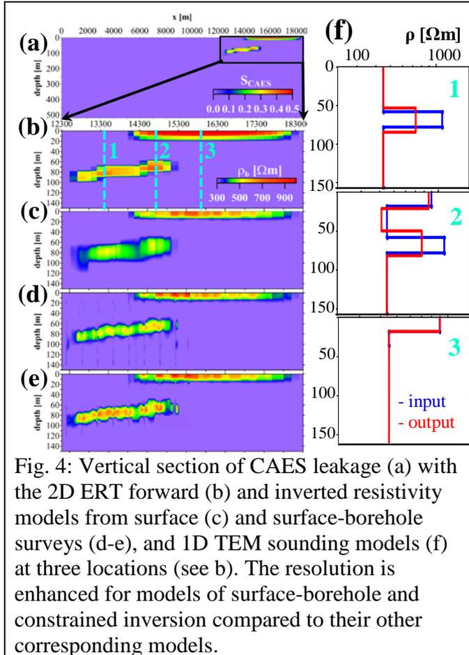
Fig. 4: Vertical section of CAES leakage (a) with the 2D ERT forward (b) and inverted resistivity models from surface (c) and surface-borehole surveys (d-e), and 1D TEM sounding models (f) at three locations (see b). The resolution is enhanced for models of surface-borehole and constrained inversion compared to their other corresponding models.
