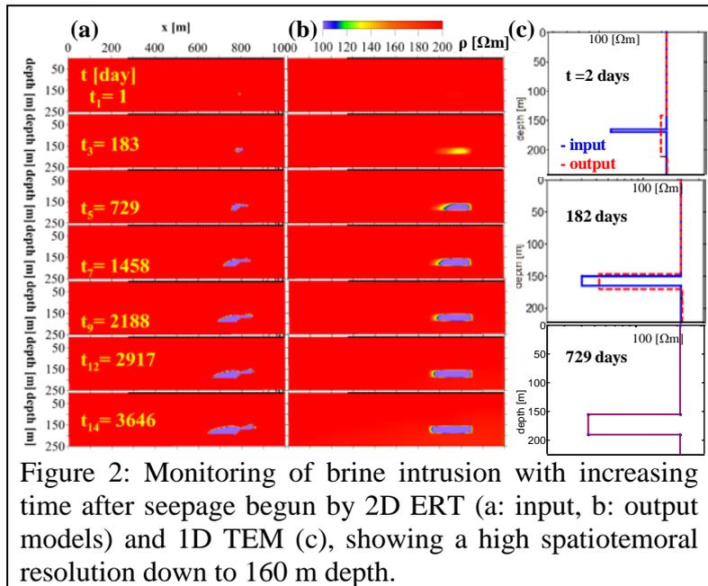
Figure 2: Monitoring of brine intrusion with increasing time after seepage begun by 2D ERT (a: input, b: output models) and 1D TEM (c), showing a high spatiotemoral resolution down to 160 m depth.
